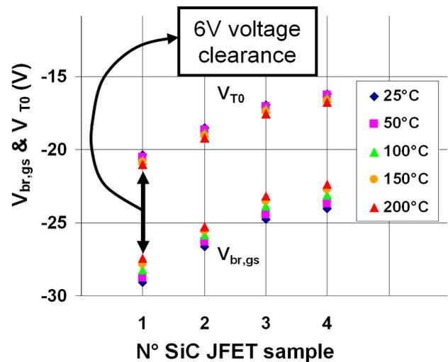
Fig. 12: Behavior of SiC JFET gates on 4 samples at temperatures up to 200°C. Top : Threshold gate-source voltage  $V_{T0}$  - Bottom : Breakdown gate-source voltage  $V_{br,gs}$
