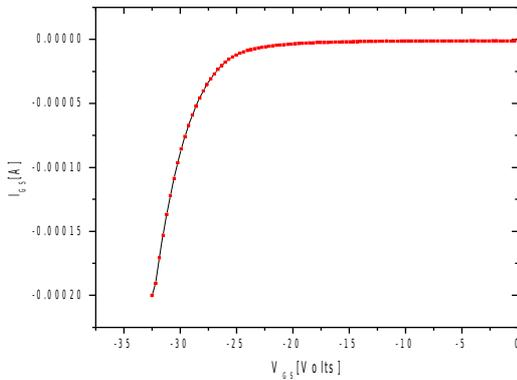
Fig. 10: Current-voltage characteristics of the gate junction in reverse mode for a SiCED-JFET (4.1 x4.1 mm<sup>2</sup>) in lot n°HY064
