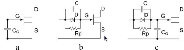
Fig. 15: Three specific SiC JFET Gate Driver Circuits
