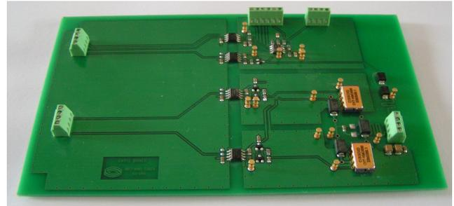
Fig. 19: Driver using SOI MOSFET technology from CISSOID
