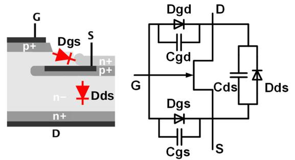
Fig. 11: SiC VJFET cross section and equivalent circuit.
