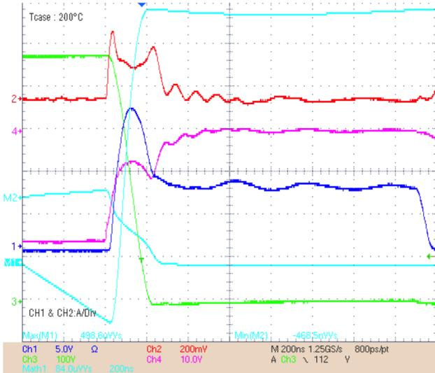
Fig. 20: Turn-on measurements during an inverter operation at 540V, 15A and 200°C
