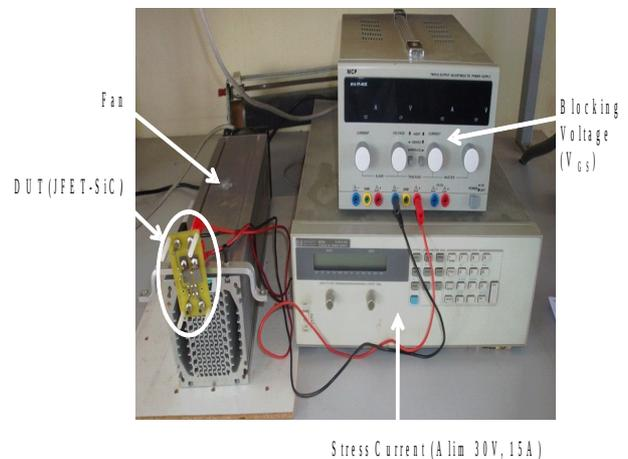
Fig. 1: test bench for measuring the degradation of a JFET
