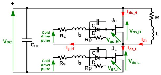
Fig. 14: Setup used to show drain-to-gate interaction
