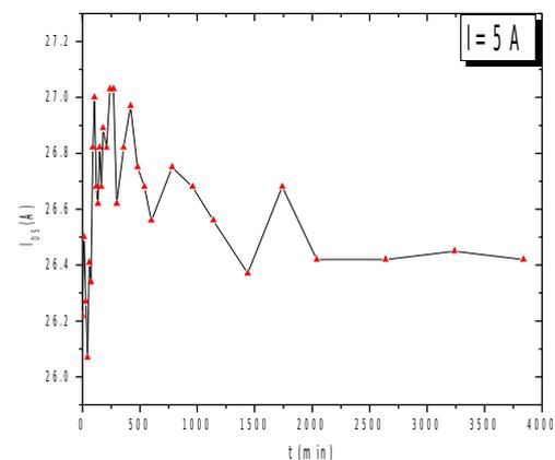
Fig. 4: Degradation of the saturation current during a 64 h stress with a 5 A reverse continuous current for a SiC-JFET form SiCED (2.4 x 2.4 mm<sup>2</sup>).
