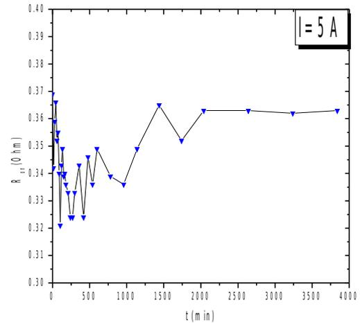
Fig. 3: Degradation of the on-resistance during a 64h stress with a 5 A reverse continuous current for a SiC-JFET form SiCED (2.4 x 2.4 mm<sup>2</sup>).
