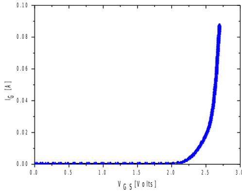
Fig. 9: Current-voltage characteristics of the gate junction in forward mode for a SiCED-JFET (4.1 x4.1 mm<sup>2</sup>) in lot n°HY064
