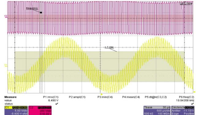
Fig. 22: line current and output voltage measurements during an inverter operation at 540V, 15A and 200°C
