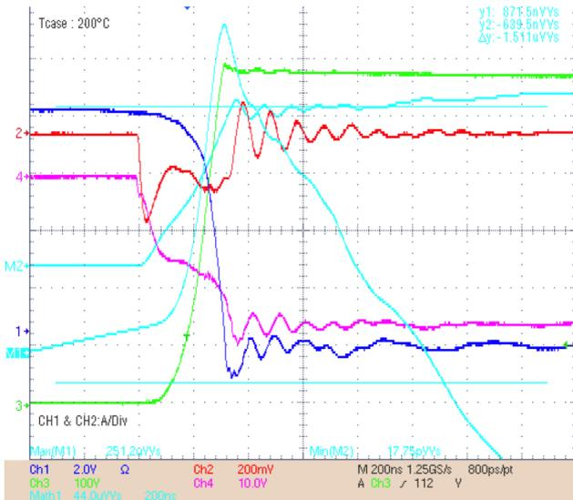
Fig. 21: Turn-off measurements during an inverter operation at 540V, 15A and 200°C
