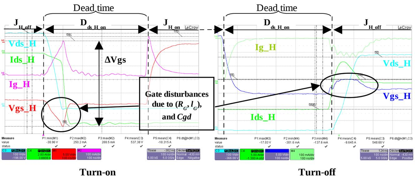
Fig. 13: Switching curves of JFET  $J_H$  working in free wheeling mode 540V on DC bus voltage, 10A switched current.  $V_{TO} = -19.2V$ , Blocking voltage =  $V_{TO}-3V$ ,  $T = 25^\circ C$ . During  $J_H$  turn-on, its gate operates in punch-through condition since  $\Delta V_{gs} \approx 31V < V_{br,gs}$ .
