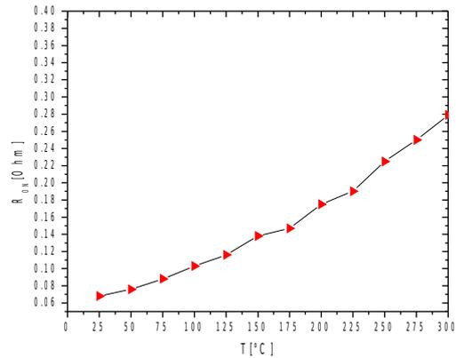
Fig. 7: On-resistance,  $R_{ON}$ , versus temperature for a SiCED JFET in lot n°HY064 (4.16 x 4.16 mm<sup>2</sup>).
