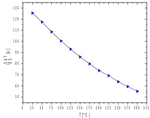
Fig. 8: Saturation current,  $I_{DS}^{SAT}$ , versus temperature for a SiCED JFET in lot n°HY064 (4.16 x 4.16 mm<sup>2</sup>).
