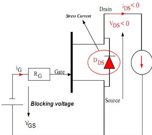
Fig. 2: Principle circuit for measuring the degradation of a JFET
