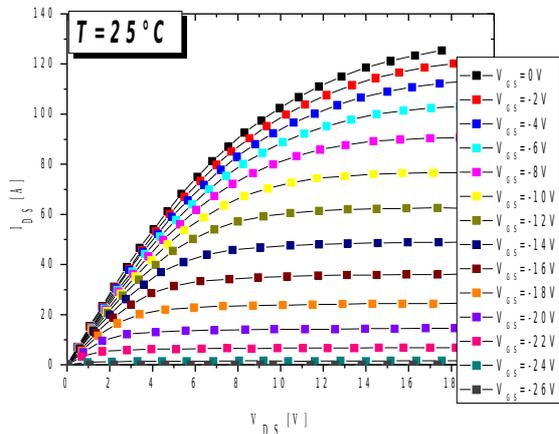
Fig. 5: Steady state characteristics in forward bias mode of the SiCED-JFET lot HY064 at room temperature (left) and at 300°C (right)
