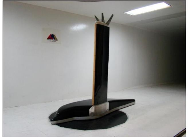
Fig. 1 Model prepared for the wing tunnel testing
