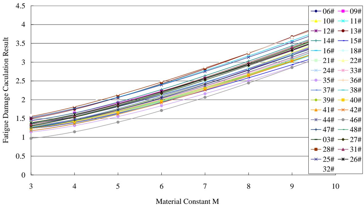
Fig .4. Fatigue Damage Calculation With Different Material Constant  $M$  for Each Aircraft Of Type B ( More than 300 hours)
