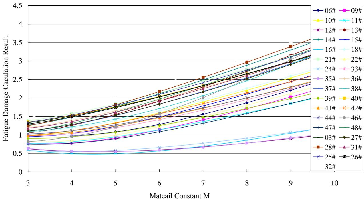
Fig. 2. Fatigue Damage Calculation With Different Material Constant  $M$  for Each Aircraft Of Type B (less than 100 hour)
