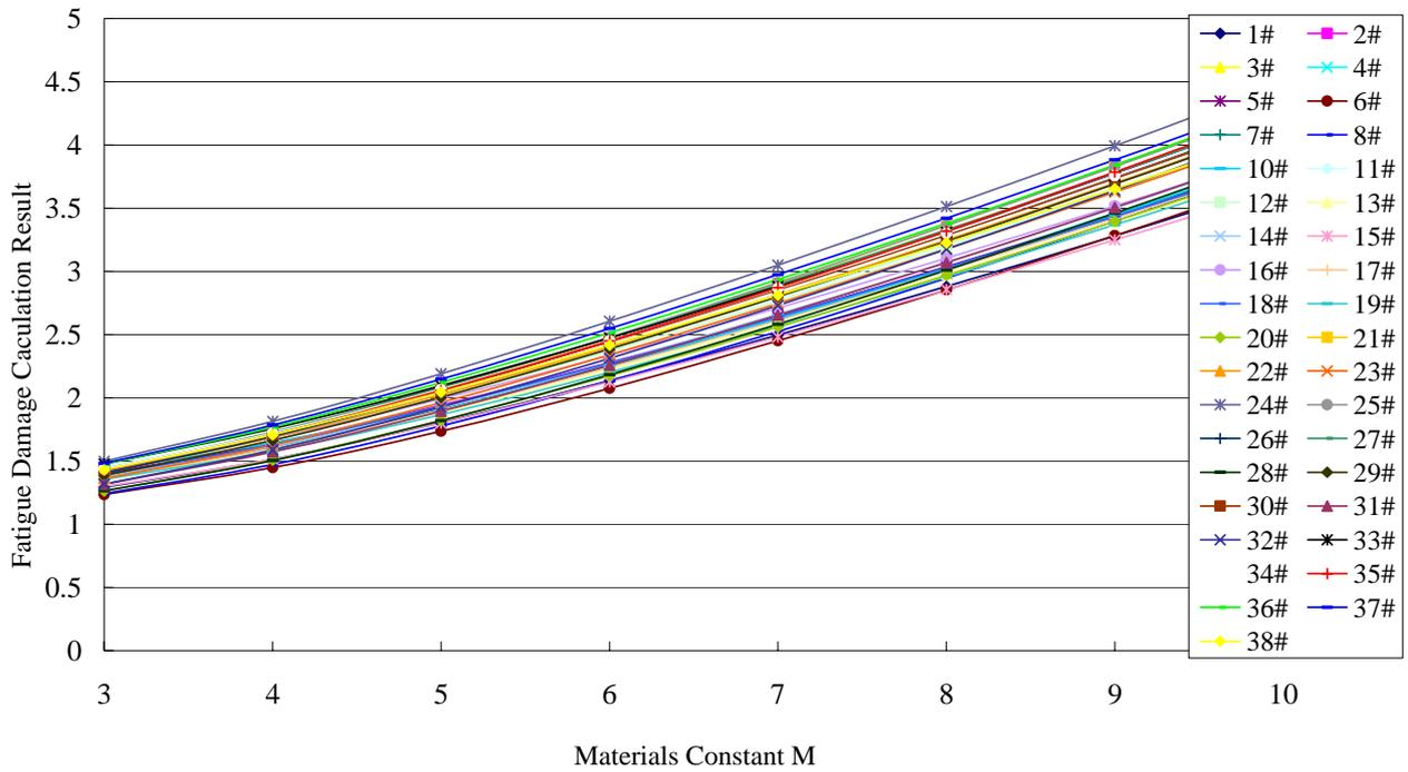
Fig.1. Fatigue Damage Calculated With Different Material Constant  $M$  ( $M=3\sim 9$ ) For Each Aircraft Of Type A
