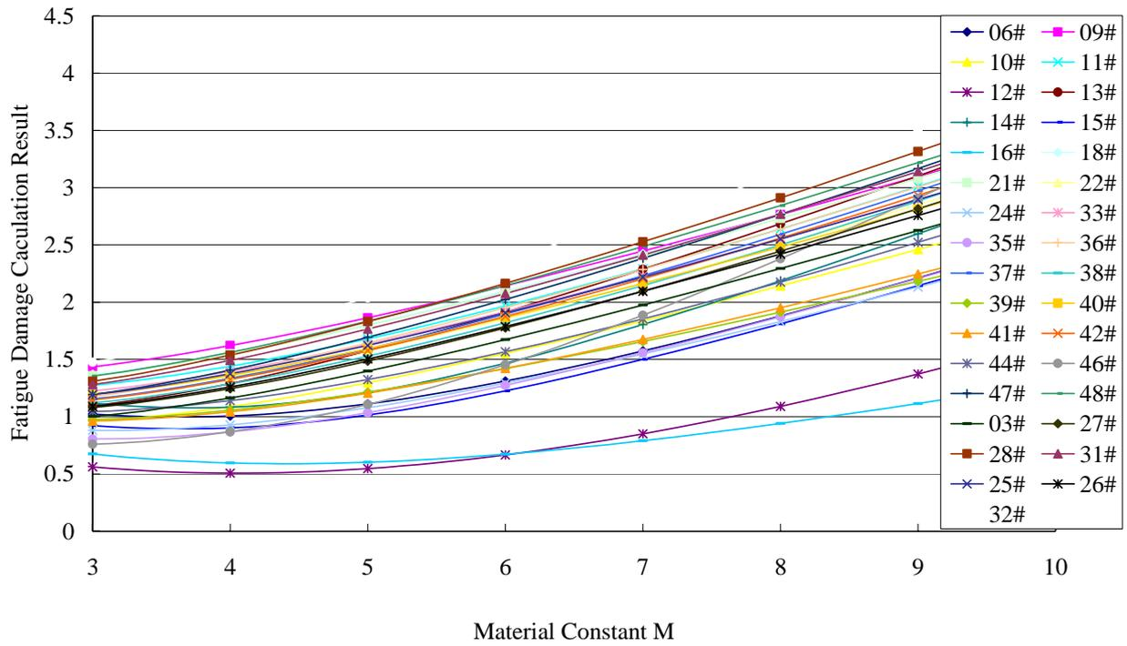
Fig 3 Fatigue Damage Calculations With Different Material Constant  $M$  For Each Aircraft Of Type A (Between 100 and 200 hours)
