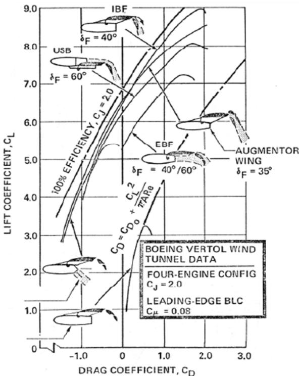
Fig. 2 depicts the different high lift systems and their maximum lift coefficient.
