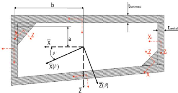
Fig. 5 depicts the profile cross section structural layout of the wing-box for the inverse calculation of I. The triangular areas are necessary to increase the moments of inertia with respect to the twisted bending moment axis.
