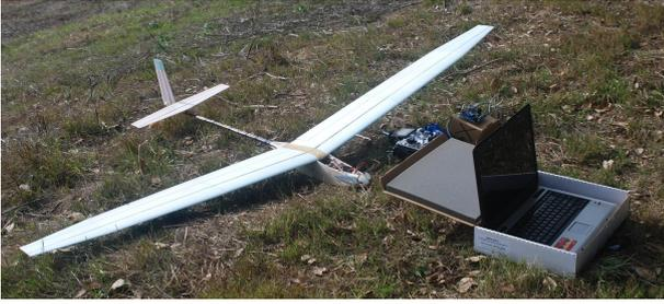
**Fig. 6** The UAV system, including the ground station.
