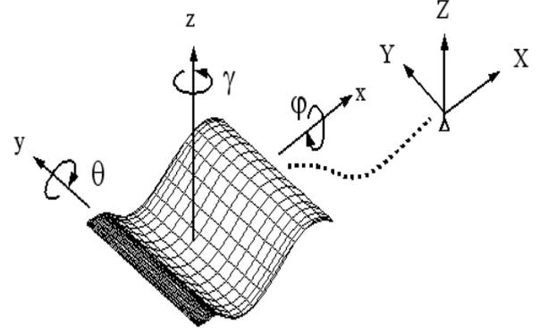
Fig. 1. Inertial and body coordinates used to describe the motion of the body
