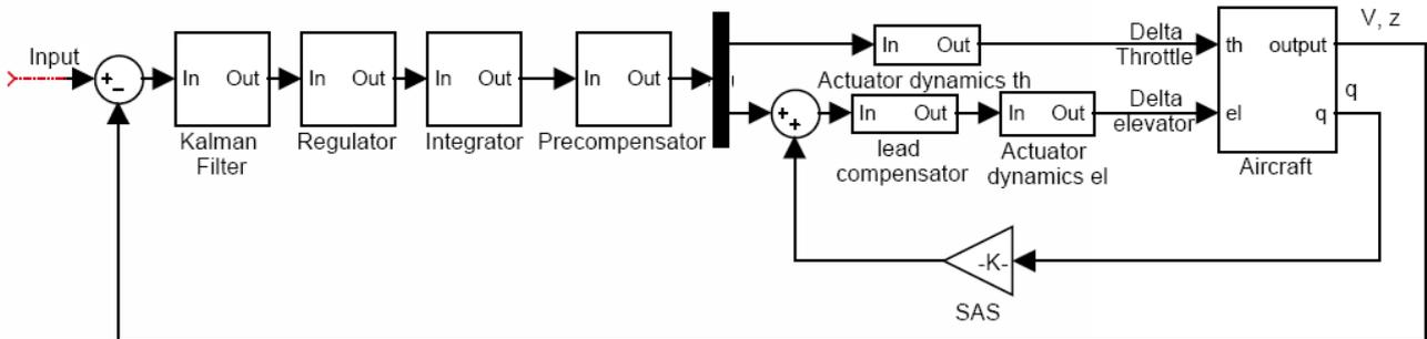
Fig.2. Controlled system architecture
