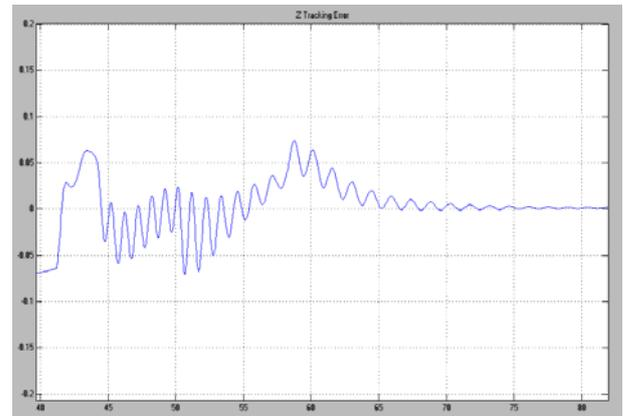
Fig.5. Altitude tracking error in landing manoeuvre
