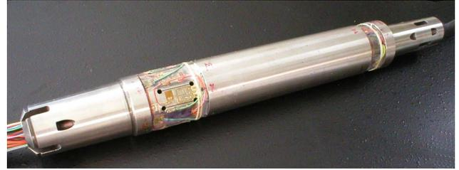
Fig. 2 Photograph of the new balance
