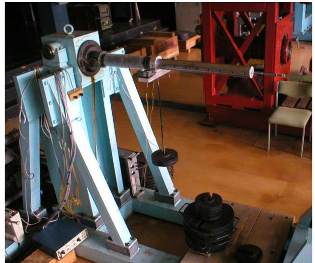
Fig. 4 Balance on the calibration rig
