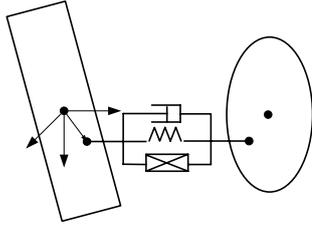
Figure 2 Spring-dampers-actuator
