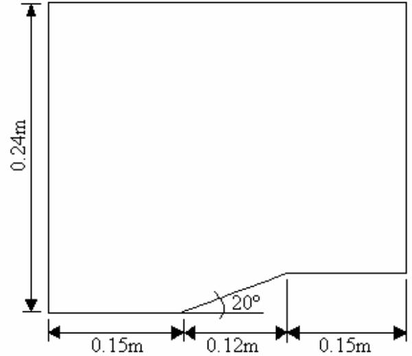
Figure 1. Ramp configuration at the xy plane.
