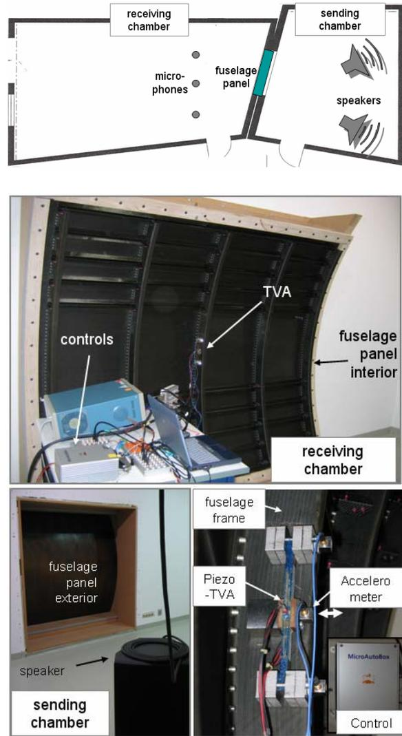
**Fig. 6** Transmission loss test suite
