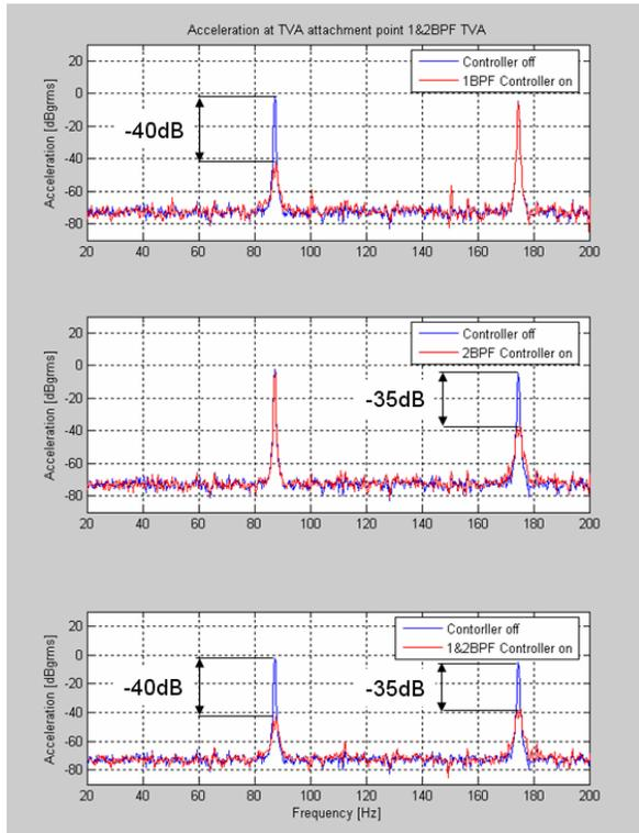
**Fig. 7** Vibration reduction of 1BPF-TVA in multi-mode operation at 655rpm
