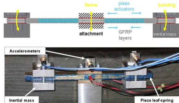
**Fig. 2** Piezo-TVA working principle and hardware realization
