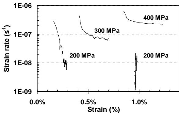
Fig. 10. Compressive creep curve in true strain rate vs. true strain representation indicating steady-state creep (i.e. constant creep rate) of a Nb-base silicide alloy at 1200°C (total test duration: 45 h).
