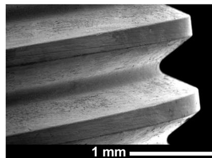
Fig. 16. Machining of the thread of a tensile test specimen (Nb-silicide alloy).
