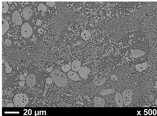
Fig. 6. SEM micrograph in backscattered electrons imaging mode (BSE) of the gas-atomised and HIP'ed Mo-Si-B alloy with Mo(ss) (bright), intermetallics (grey) and silica (dark).
