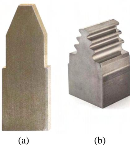
Fig. 14. Precision machining of Mo-base silicide alloy: from the preform (a) to the firtree mockup (a; height is about 25 mm).
