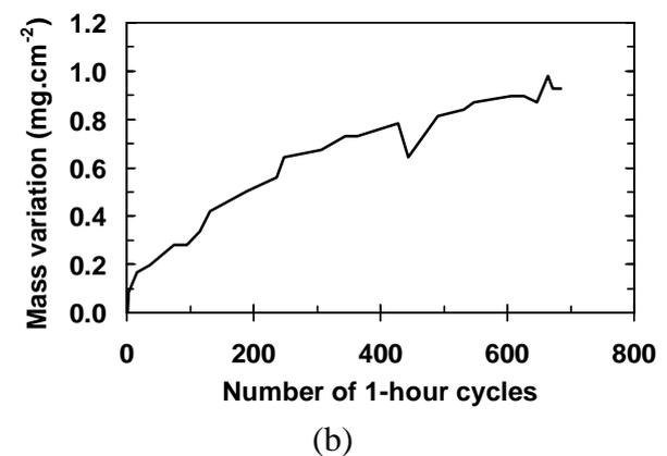
Fig. 13. Cyclic oxidation at 1100°C of coated Mo-base alloy. Coating based on Fe-Cr-Si (a) and SIBOR<sup>®</sup> coating based on Mo-Si-B (b).
