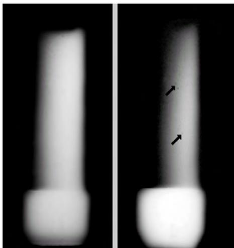
Fig. 5. X-ray radiographs with different exposure time of the same blade, showing reduced casting defect level (pores are shown by arrows).
