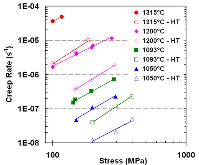
Fig. 11. Steady-state creep rate vs. stress for the HIP'ed (full symbols) and heat-treated (1700°C, 10 h; open symbols) MoNbSiB alloy for temperatures between 1050°C and 1315°C.
