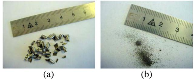
Fig. 15. Shavings from (a) Nb-base and (b) Mo-base silicide alloys.
