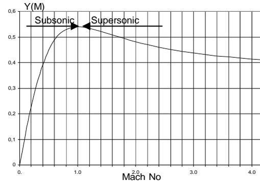
**Fig.6.** The shorthand  $Y(M)$  as a function of the Mach No.
