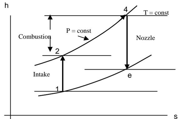
**Fig.2.** The ideal ramjet in an enthalpy (h) – entropy (s) diagram
