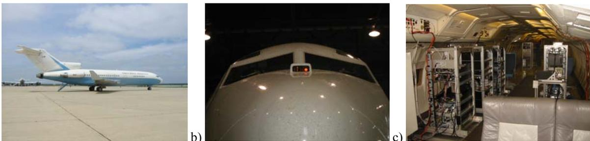
Fig. 1. SE-Vision Project. a) FAA’s Test Aircraft Boeing 727 on Atlantic City Airport, b) Max-Viz IR-Camera System, c) Installed Flight Test Equipment.
