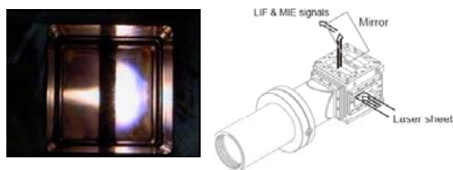
Fig. 15. Lund LTH rig. Normal photograph of the flowfield (left) ; LIF/MIE measurement (right)
