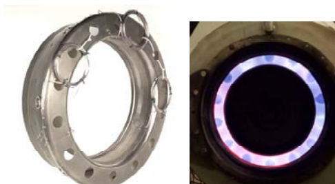
Fig. 23. LPP return bend combustor and TM P0 tests
