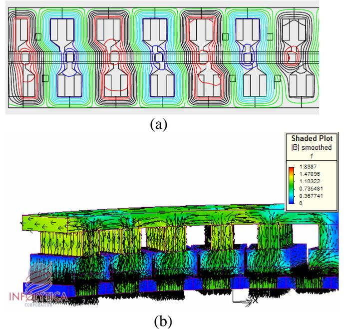
**Fig 5.** (a) The equi-potential lines, magnetic vector potential. (b) The flux density taking the fringing effects into account
