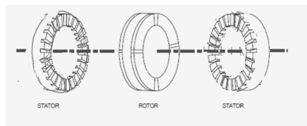
**Fig 1.** A four pole axial flux machine with rotor and a double stator assembly
