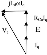
**Fig 4.** Phasor diagram, motor operation
