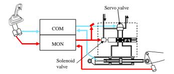
Fig. 1b. Computer Monitoring Architecture
