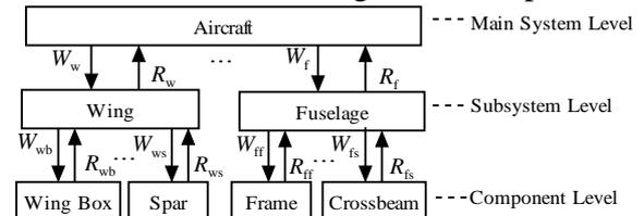
Fig. 14 Simplified weight requirement allocation architecture for aircraft structure
