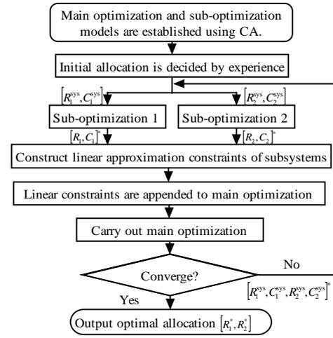
Fig. 4 Flowchart of optimum allocation in Eq.3 using CA
