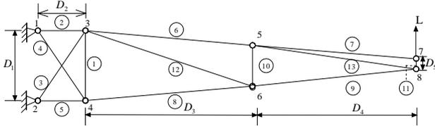
Fig.11 Topology of the engineering truss
