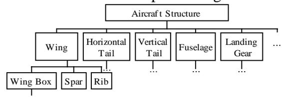
Fig. 1 Hierarchical decomposition framework of aircraft
