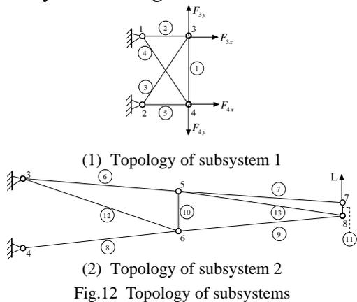
Fig.12 Topology of subsystems
