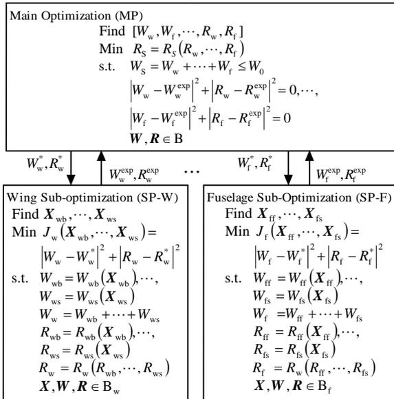
Fig. 15 Mathematical model of weight requirement collaborative allocation according to Fig.14
