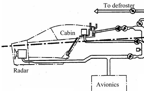
Fig. 7 Schematic view of the distribution sub-system in the ECS in Gripen.
