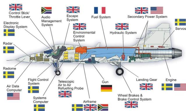
Fig. 2 The system layout in Gripen
