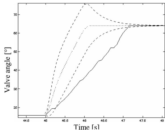
Fig. 8 A jamming valve. Measured angle (solid), estimated angle (dotted) and its adaptive thresholds (dashed).
