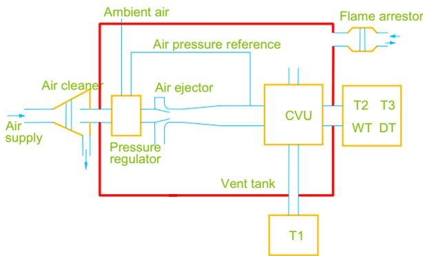
Fig. 9 Schematic view of the tank ventilation and pressurization system in Gripen.
