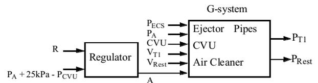
Fig. 10 The G-system that is modeled by system identification.
