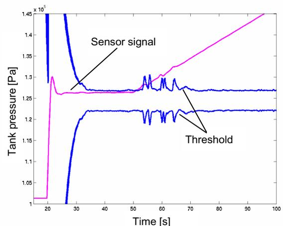
Fig. 11 Example with an incipient fault in a pressure sensor after 50 s.
