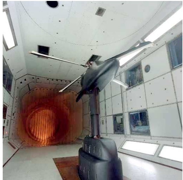
Rotor test rig and experimental rotor in QinetiQ 5 Metre Wind Tunnel, from HC(AG) on 'Validation of Rotor / Hub Load Synthesis Techniques'
