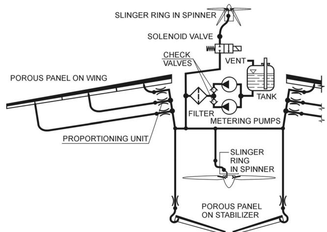
Fig.12 Ice Protection Fluid System proposed for MALE UAV, developed at Warsaw University of Technology
