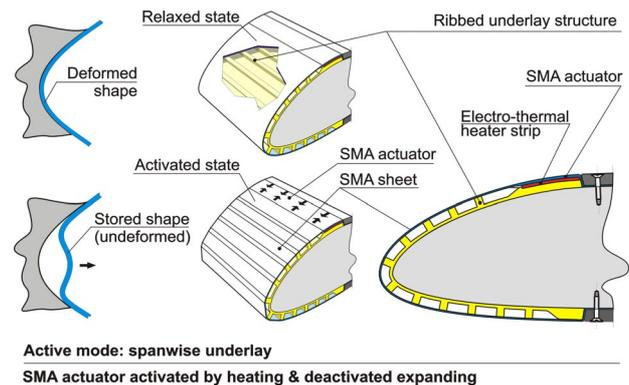
Fig.13 Ice Protection System based on Shape Memory Alloys, US Patent 5,686,003
