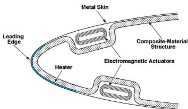
Fig.4 Electro-Expulsive Deicer located in the wing nose – a possible arrangement
