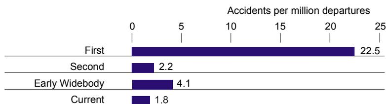
Fig.2 Accident categories by airplane generation, all accidents, worldwide commercial jet operations, 1990-1990 , after Commercial Aviation Safety by Aviation Week, 2001 [1]
