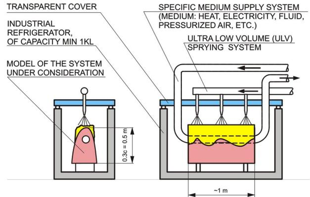
TEST STAND FOR COMPARISON OF DIFFERENT ANTI-ICING SYSTEMS
