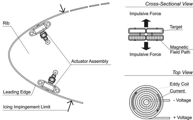
Fig.7 Impulsive coil in a leading edge (Eddy current)
