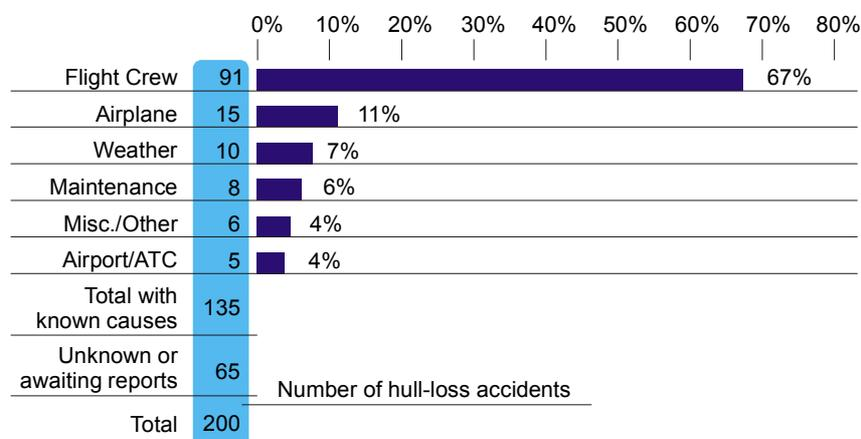
Fig.1 Primary cause factors in hull-loss accidents, all airplanes, worldwide commercial Jet fleet, 1990-1999, after Commercial Aviation Safety by Aviation Week, 2001 [1]
