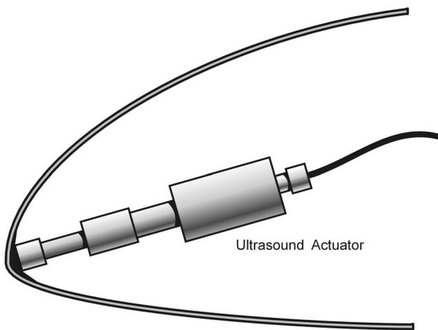
Fig.11 Ultrasound actuator placed inside the nose of leading edge
