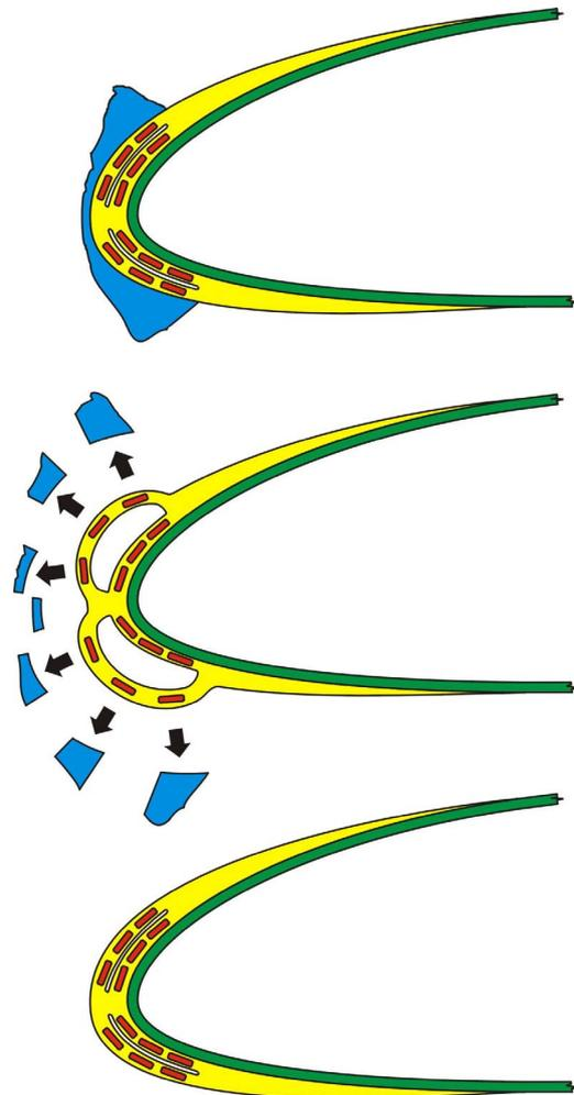
Fig.8 Ice shattering using the Electro-Expulsive Separation System
