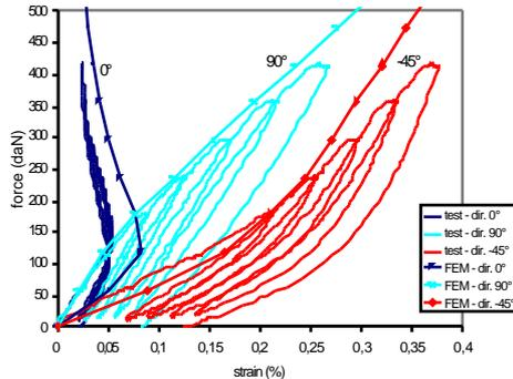
When introducing damage effects, it is possible to obtain a more realistic CMC behavior, taking into account damage history and permanent strains, as shown on fig. 18, for an unidirectional gauge at the center of the plate. In this case and concerning A500, sub-element analysis validates the identification of both coupling parameters and damage kinetics of ODM behavior law.
