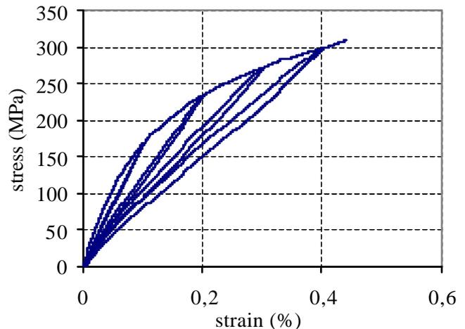
As already mentioned by other researchers [4], three domains can be observed: a linear elastic portion, a non-linear elastic domain due to microcracking starting at a macroporosity level followed by a quasi linear domain due to microcracking at the tow level. Residual strain after loading and hysteresis loops is negligible which is typical of a damageable linear elastic behavior.
