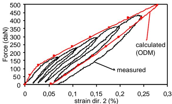
In a second time, the same sub-element had been tested under torsion loading at 873 K in air, as shown on Fig. 19. The plate was simply supported on two adjacent sides and a deviation equal to 10% of the transversal size was applied on the opposite corner. Testing was performed
