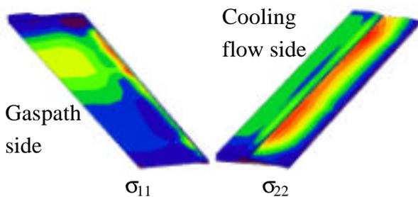
**Fig. 11** Longitudinal stress - A410 and A500 cases
