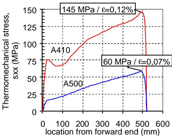
The lower sensitivity to thermal gradients of SEPCARBINOX<sup>®</sup> A500 compared with A410 is a way to increase its design margins as outlined by the following example : referring to the same design case, Fig.11 shows max. longitudinal stresses respectively of 60 MPa and 145 MPa for A500 and A410 materials. The relevant stress allowable for a
