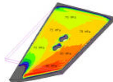
**Fig. 21** Calculated and measured strain, at RT and dir. 45° for torsion testing
