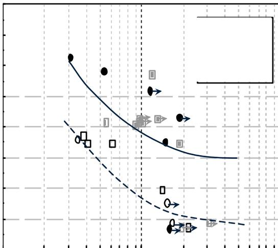
A comparison of the SEPCARBINOX® A500 behavior tested in tensile fatigue at 0.25 Hz and in tensile creep is provided in figure 8. The life time duration, in tensile fatigue, is around 100 hrs for a stress level closed to 160
