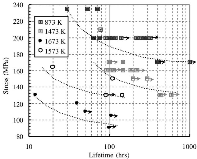
Fig. 8 A500 T/T fatigue and tensile creep, in air
