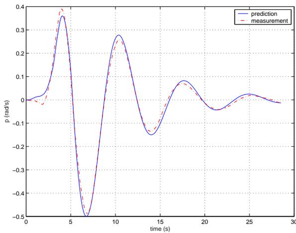
**Fig. 8** Measured roll velocity  $p$  and estimated values.
