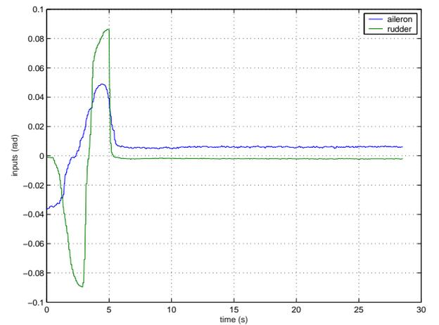
**Fig. 6** Aileron  $\delta a$  and rudder  $\delta r$  inputs for the dutch-roll maneuver.
