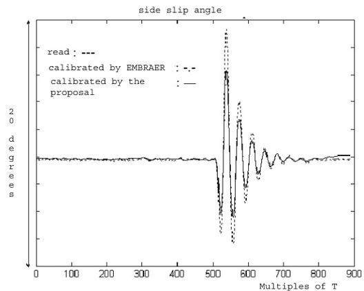
**Fig. 5** Measured and calibrated values for the side slip angle.
