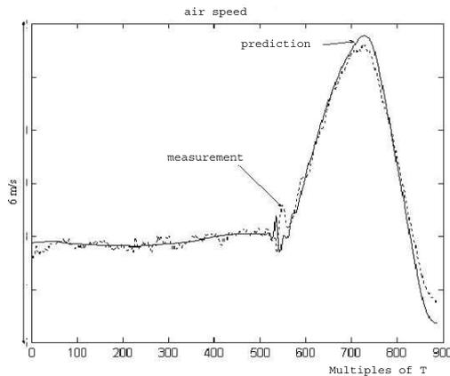
**Fig. 3** True air speed: measurements and prediction.
