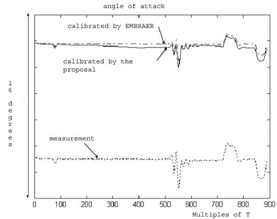
**Fig. 4** Measured and calibrated values for the angle of attack.
