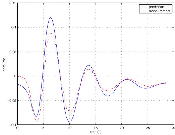
**Fig. 7** Measured side slip angle  $\beta$  and estimated values.
