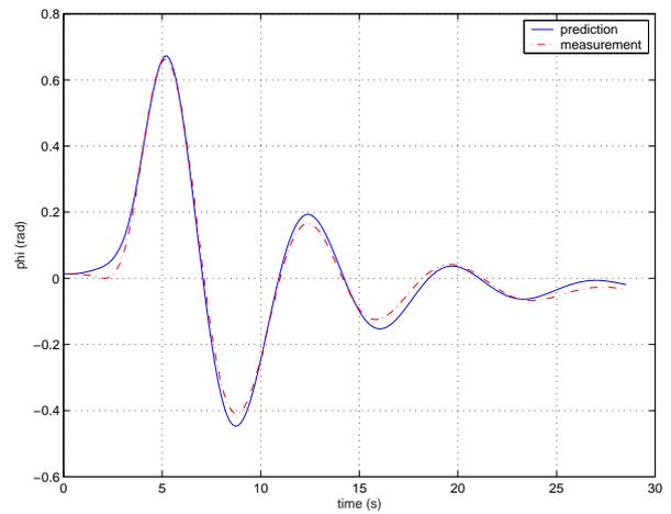
**Fig. 10** Measured bank angle  $\phi$  and estimated values.
