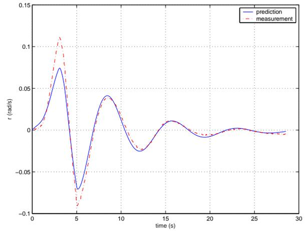
**Fig. 9** Measured yaw velocity  $r$  and estimated values.
