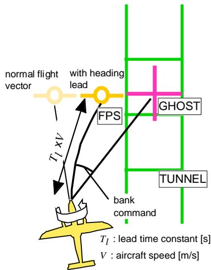
Fig. 1 Horizontal geometry of the display
