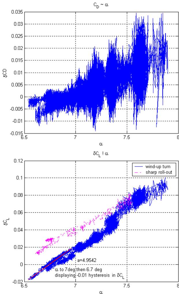
Figure 9 – buffet characteristics, medium rate turning flight manoeuvre;  $\alpha, \beta, \phi$  (deg),  $N1$  (%),  $a_x$  ('g'),  $\partial\theta/\partial t, \partial\alpha/\partial t$  (deg/sec):  $P_a=42,576\text{ft}$ ;  $M=0.630$ ;  $Rec=9.72 \times 10^6$ ;  $W=33,519\text{lb}$ ; medium rate turn;  $\alpha_B=7.2^\circ$  at  $[q \partial\alpha/\partial t]=[0.4 \ 0]$
