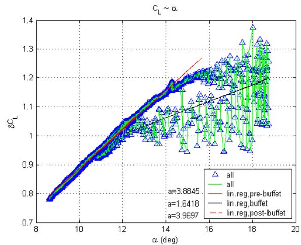
(b) lift curve with  $\alpha$ : before ( $a=3.005$ ) (auto-slat extension at  $\alpha=14.3^\circ$ ), during buffet ( $a=1.642$ ) and post-buffet ( $a=3.970$ , lower incidence); greater buffet hysteresis on reducing incidence compared to Fig.1 stalling manoeuvre.
