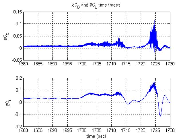
(b)  $C_L$  and  $C_D$  timetraces.
