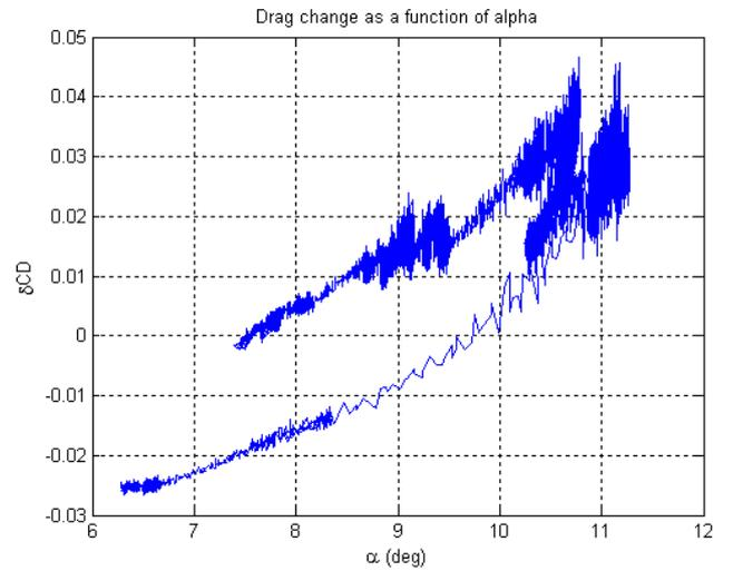
Figure 7 – buffet characteristics, further step turning flight manoeuvre, pt.1;  $P_a=32,820\text{ft}$ ;  $M=0.527$ ;  $Re_c=13.50 \times 10^6$ ;  $W=28,717\text{ lb}$ ; steep turn;  $\alpha_B=8.5^\circ$  at  $|q \frac{\partial \alpha}{\partial t}|=[2.8 \ 0]$ ; and  $\alpha_B=8.1^\circ$  at  $|q \frac{\partial \alpha}{\partial t}|=[2.65 \ 0]$ .
