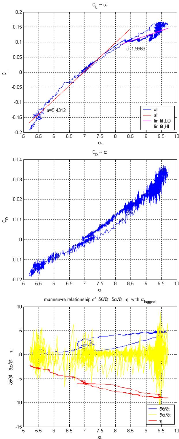
Figure 6 – buffet characteristics in a steep turning flight manoeuvre  $\sim \alpha$  (deg);  $P_a=31,190\text{ft}$ ;  $M=0.578$ ;  $Rec=15.67 \times 10^6$ ;  $W=28,717\text{ lb}$ ; steep turn;  $\alpha_B=8.3^\circ$  at  $|\dot{\alpha}/\delta t|=|4\ 0.3|$ .
