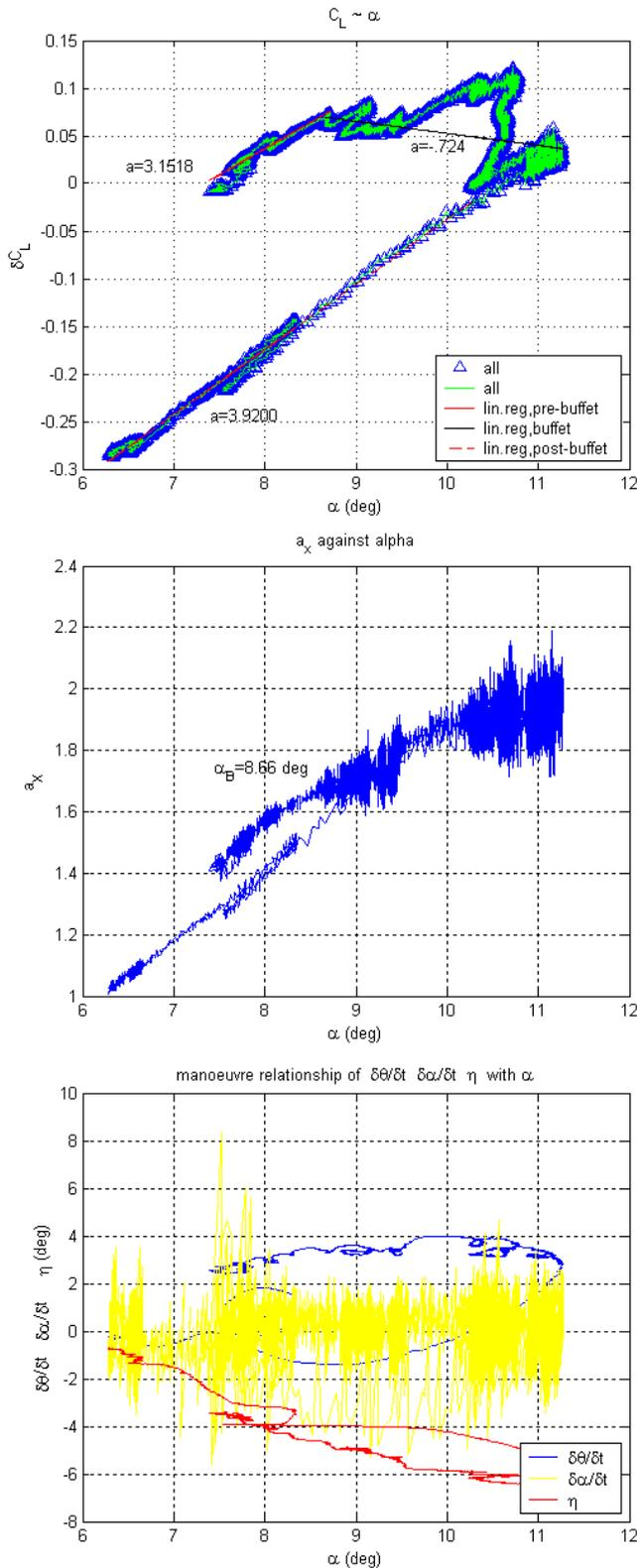
Figure 8 – buffet characteristics, further steep turning flight manoeuvre, pt.2: initial  $\alpha=7.5^\circ$ , final  $\alpha=6.3^\circ$ ;  $\alpha, \beta, \phi$  (deg),  $N1$  (%),  $a_x$  ('g'),  $\partial\theta/\partial t, \partial\alpha/\partial t$  (deg/sec);  $Pa=32,820ft$ ;  $M=0.527$ ;  $Rec=13.50 \times 10^6$ ;  $W=28,717$  lb; steep turn; steep turn;  $\alpha_B=8.66^\circ$  at  $[q \partial\alpha/\partial t]=[3.5 \ 0.5]$ .
