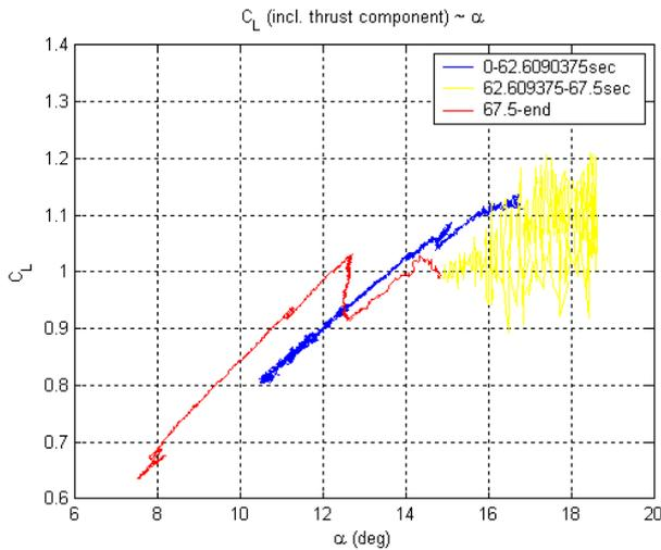
(b) lift curve with  $\alpha$ : before ( $a=3.301$ ) (auto-slat extension at  $\alpha=15^\circ$ ), during buffet ( $a=1.697$ ) and post-buffet ( $a=4.554$ , lower incidence) (auto-slat retraction at  $\alpha=14.7^\circ$ , thrust advance at  $\alpha=12.6^\circ$ ).
