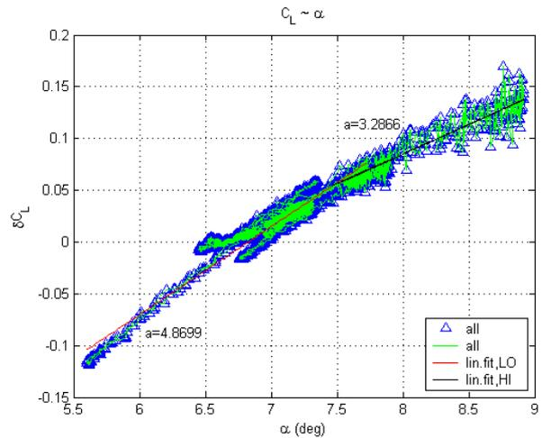
(a)  $C_L$  characteristics; in buffet, a 33% loss of lift curve slope occurred.
