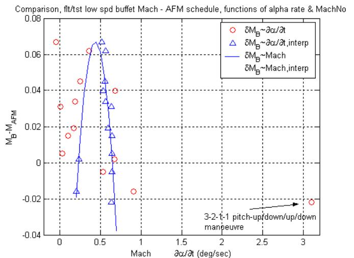
Figure 11 – comparison of low-speed buffet onset Mach Number with flight manual scheduled data.
