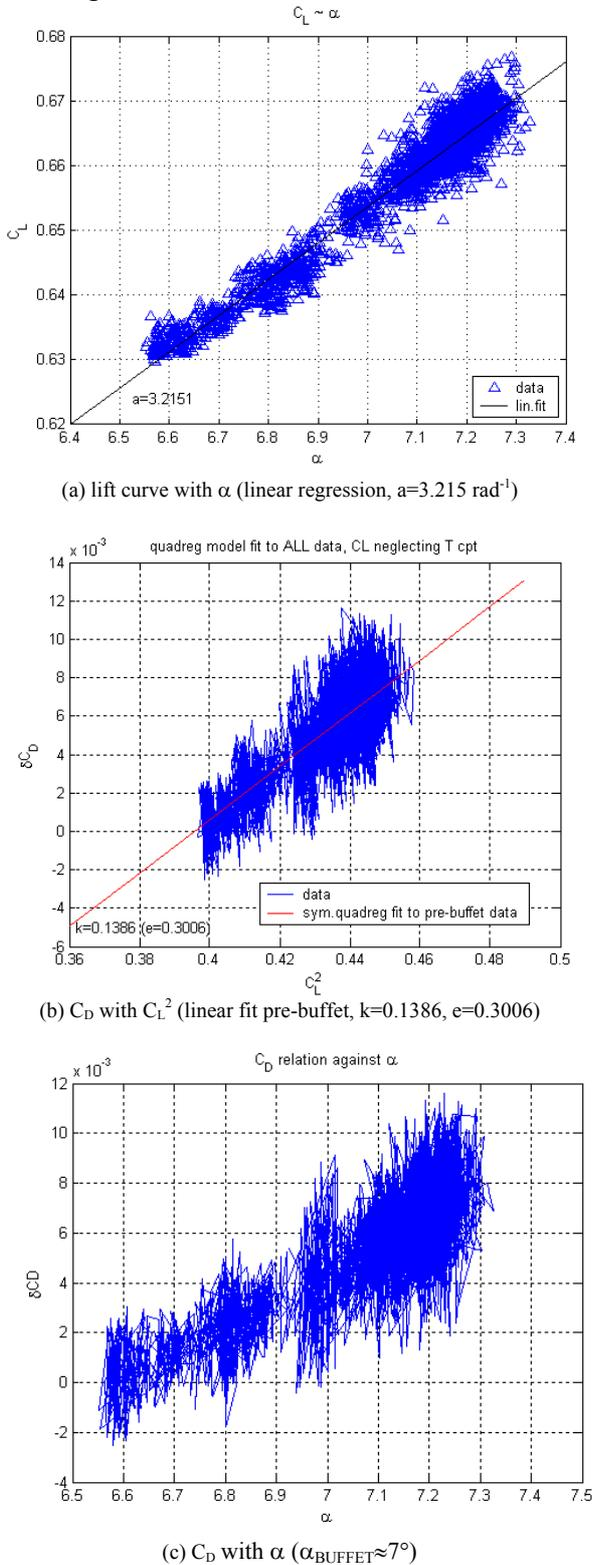
Figure 3 – buffet characteristics, straight and level flight.  $\text{Pa}=43,000\text{ft}$ ;  $M=0.638$  ;  $\alpha_B=6.95^\circ$  at  $[q \partial\alpha/\partial t]=[0 \ 0] \text{ s}^{-1}$
