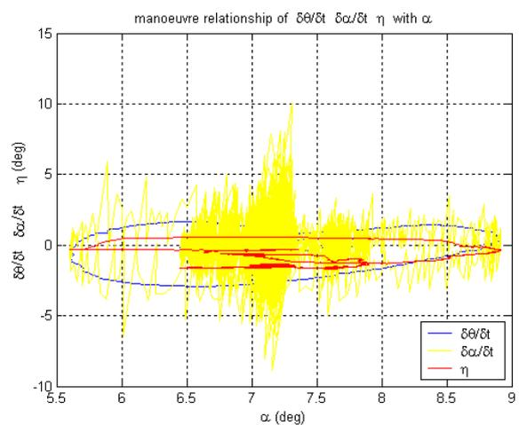
(c) maps of incidence and pitch rates (deg/sec) and elevator angle (deg) maps with  $\alpha$
