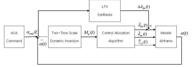
Fig. 1 Angle of attack tracking control system
