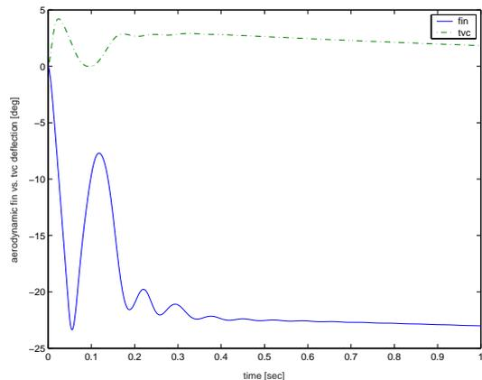
Fig. 5 Distributed aerodynamic fin vs. thrust vectoring control for Scenario 1
