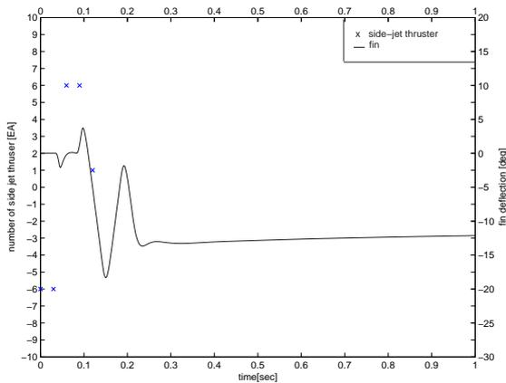
**Fig. 7** Distributed aerodynamic fin vs. side-jet thrust control for Scenario 2
