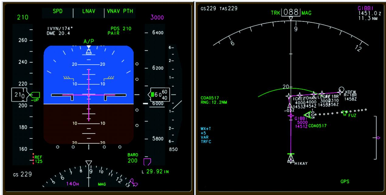
**Fig. 5** Primary Flight Display (PFD) and Navigation Display (ND) of the Boeing 777-like simulator with AMSTAR/Pair Dependent Spacing symbology. The PFD shows the PDS annunciation in the upper right corner under the Flight Mode Annunciator and the commanded speed on the speed tape. The ND shows the lead aircraft highlighted in green along with history dots. Note that the aircraft is approaching a merge point with the lead aircraft.
