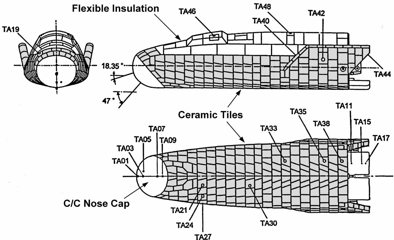
Fig. 4. HYFLEX TPS and Temperature Measurement Locations
