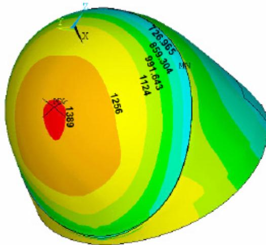
Fig. 7. Comparisons of Nose Temperature with and without Inner Radiation Effect
