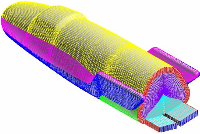
Fig. 11. Surface Mesh for Base Flow Calculation
