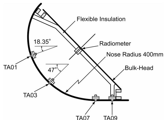
Fig. 5. C/C Nose Cap Temperature Measurements Points
