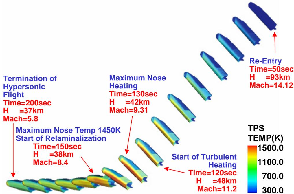
Fig. 1. HYFLEX Re-Entry Flight Simulation Representing TPS Surface Temperature Change at 10 sec Intervals in Hypersonic Speed Range
