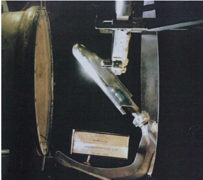
Fig. 8. HYFLEX 10 % Scale Model Setting in ONERA F4
