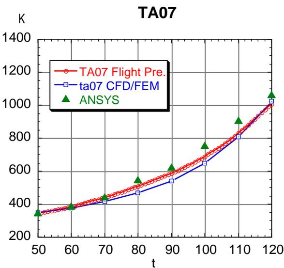
Fig. 6. Comparisons of Temperature Increase of HYFLEX C/C Nose Cap with Flight Data
