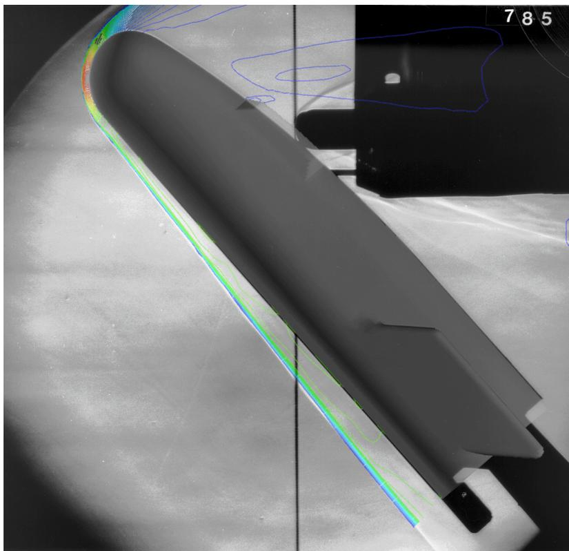
Fig. 9. Comparison of Shock Wave Shape with Schrielen Photograph in ONERA F4
