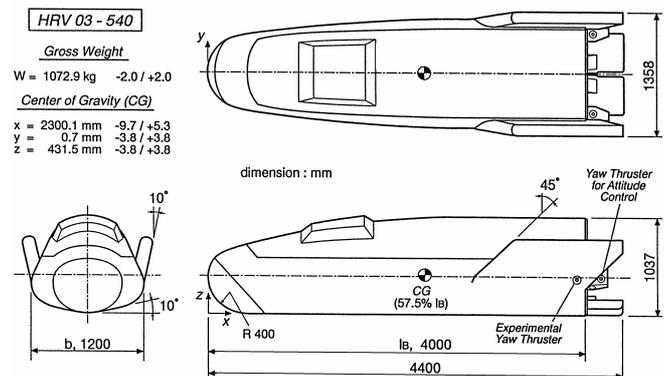
Fig. 2. HYFLEX Vehicle Configuration
