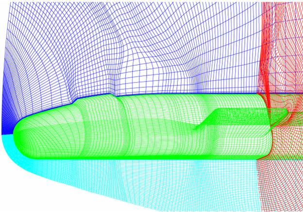
Fig. 3. CFD Grids for Outer Flow Calculations (101x89x61)
