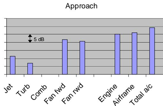
Fig. 1. Noise sources for a generic quad engine long-range aircraft at take-off and approach conditions. Airframe noise includes wings and landing gear noise. Engine noise includes Jet, Turbine, Combustion, fan forward and fan rearward components.
