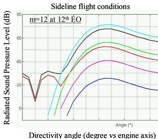
Fig. 6. Acoustic radiation of 12th azimuthal mode at 12th EO frequency at Sideline conditions.
