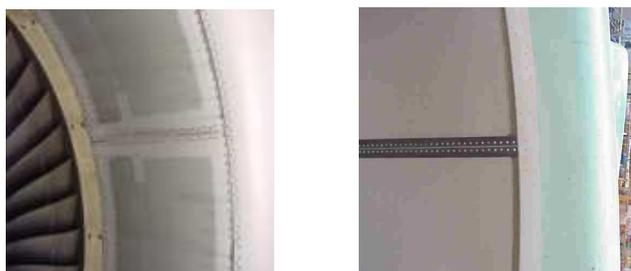
Fig. 2. 3 wide splices liner for A320 engine intake (left) and 2 narrow splices liner for A340-500/600 intake (right).
