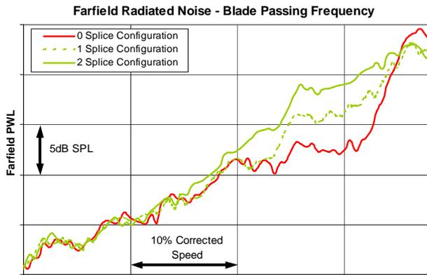
Fig. 5. 1/3 scale fan rig tests of splice effects on radiated forward noise. 1st Blade Passing Frequency fwd noise vs engine speed.
