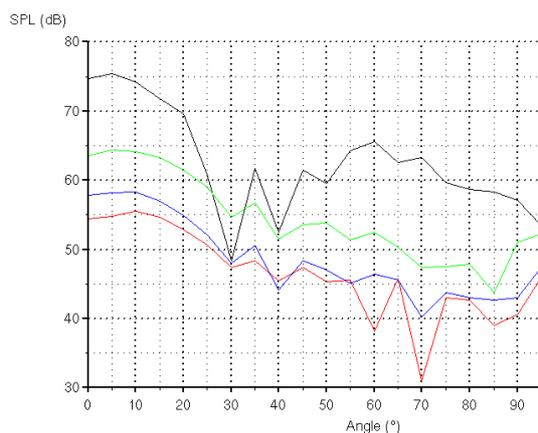
Fig. 4. No-flow tests of splice effects on radiated forward noise ( $kR=4$ ). — Hardwall duct. — 1 circumferential splice liner. — A340-500/600 style 2 axial splices liner. — 0 splice liner.
