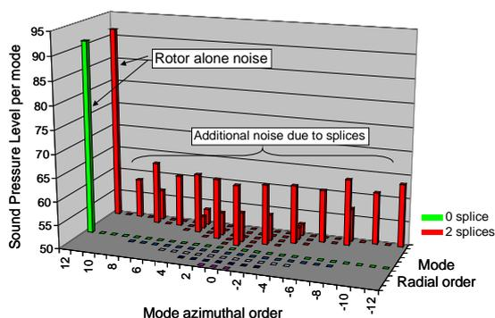
Fig. 3. Induct noise for a 2 splices (red) and a 0 splice (green) intake liner configurations.
