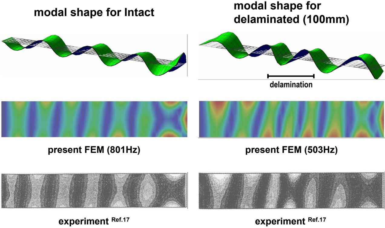
Fig.9. Modal shapes ('bending-only' 8<sup>th</sup> mode)
