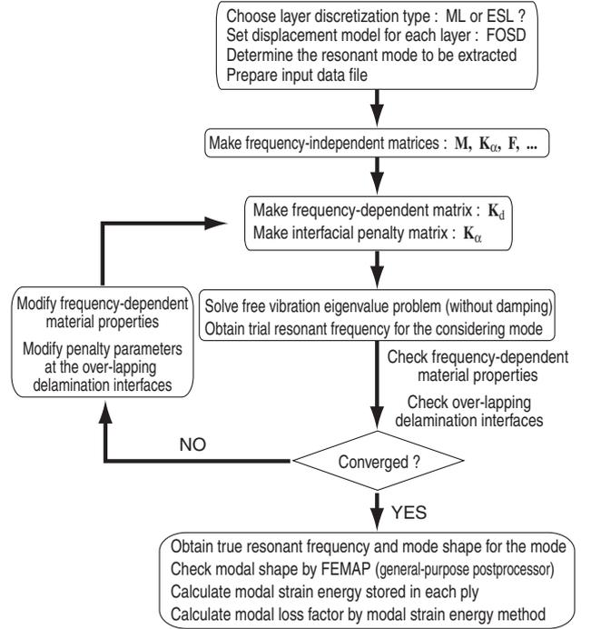
Fig.3. Program flow chart of the present non-linear iterative finite element free-vibration eigen-value analysis.
