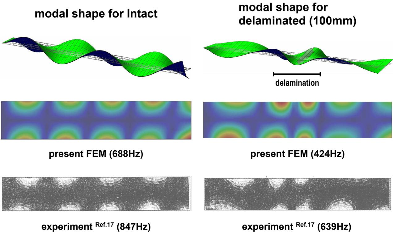
Fig.10. Modal shapes ('bending-with-torsion' 5<sup>th</sup> mode)
