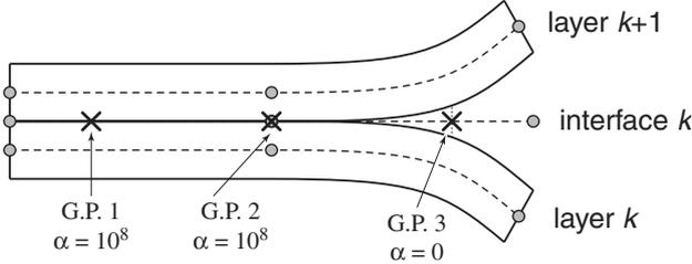
Fig.2. Adhesion and delamination modelings by the penalty function method.
