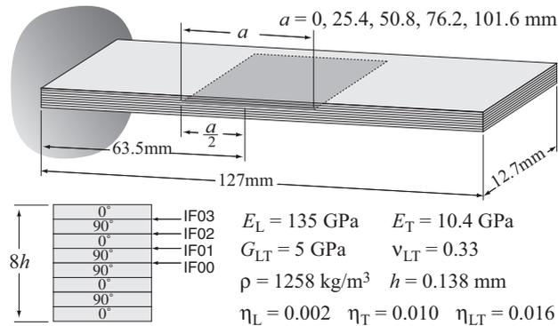
Fig.4. Delaminated CFRP cross-ply cantilever beams (Shen & Grady<sup>Ref.8</sup>).
