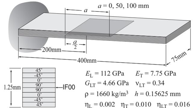
Fig.7. Delaminated CFRP quasi-isotropic beams (Kimpara *et al.* Ref.17).
