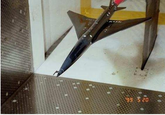
**Fig. 1** 8.5% scaled model of NEXST-1
