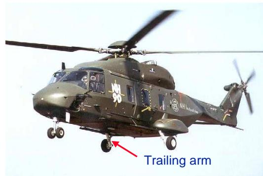
Figure 9: Location of the trailing arm in the main landing gear.
