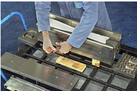
Figure 4: Positioning the pre-form and core mandrel into the inner mould.
