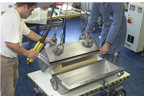
Figure 5: Positioning the inner mould (including pre-form and core mandrel) into the outer mould.
