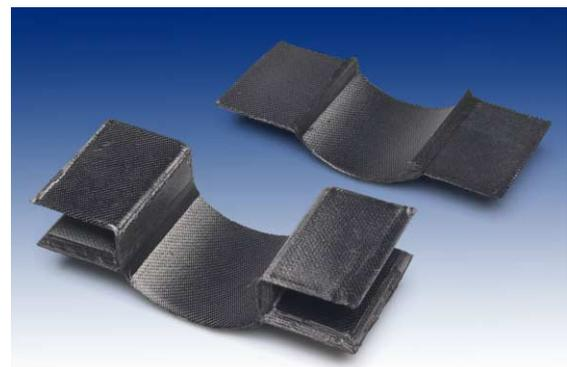
Figure 12: Net-shaped preforms for the lug area of the trailing arm using binder technique.
