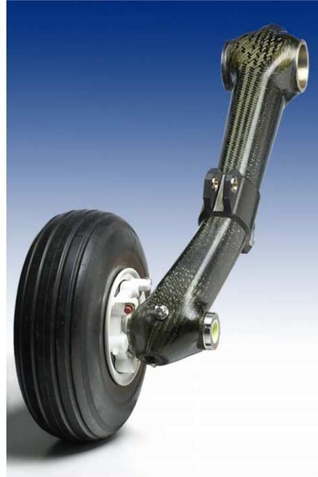
Figure 13: Composite trailing arm after assembly of the steel wheel axle and the wheel.
