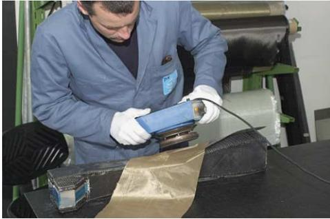
Figure 3: Making the pre-form on the core mandrel.
