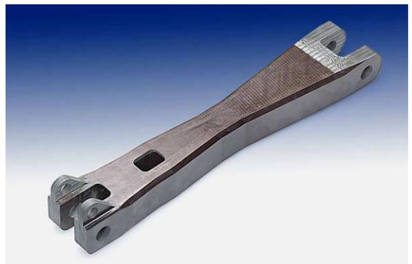
Figure 6: Cured composite drag brace after machining the lugs.
