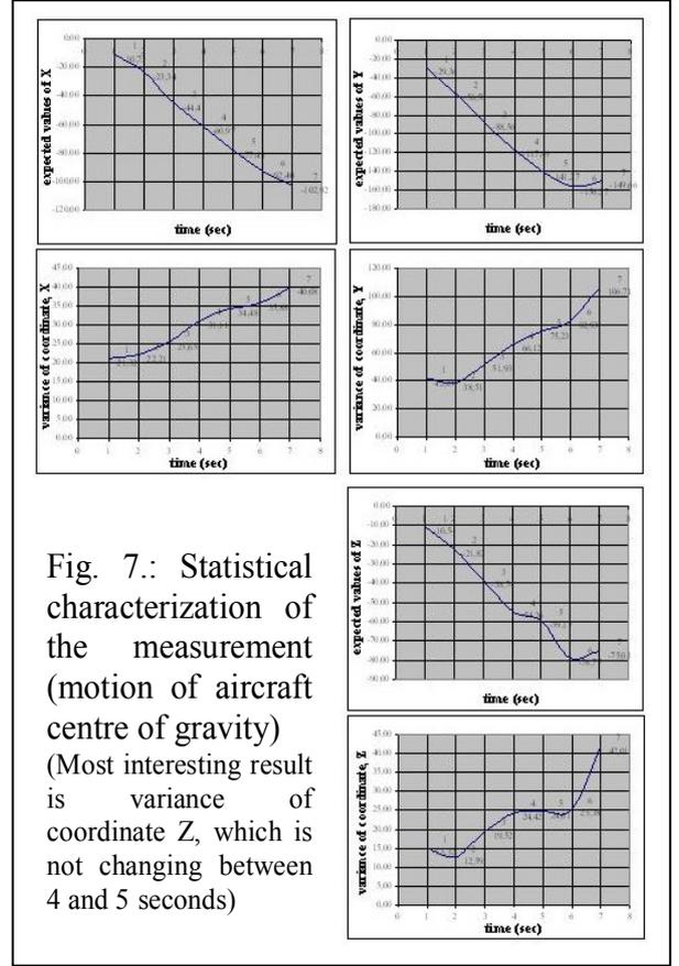
Fig. 7.: Statistical characterization of the measurement (motion of aircraft centre of gravity) (Most interesting result is variance of coordinate Z, which is not changing between 4 and 5 seconds)
