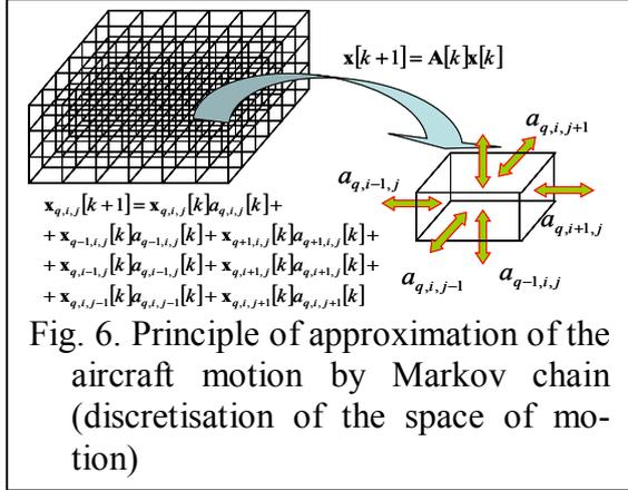
Fig. 6. Principle of approximation of the aircraft motion by Markov chain (discretisation of the space of motion)
