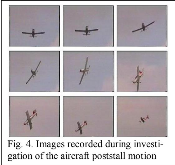
Fig. 4. Images recorded during investigation of the aircraft poststall motion
