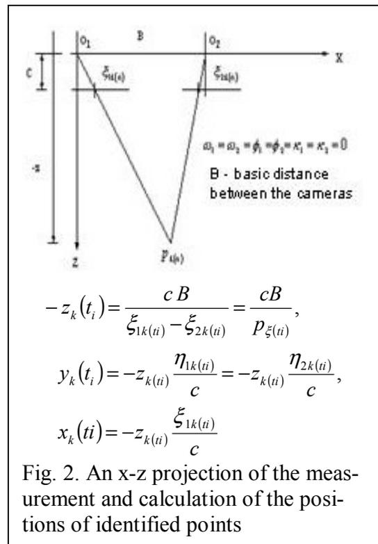
Fig. 2. An x-z projection of the measurement and calculation of the positions of identified points
