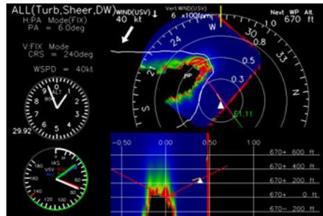
Fig. 2.2.5 Display image of 3D turbulence information.
