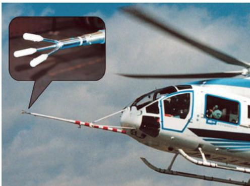
Fig. 2.1.1 Ultrasonic velocimeter installation.
