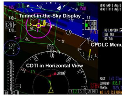
Fig. 4.2.1 Display image of 4D guidance system.
