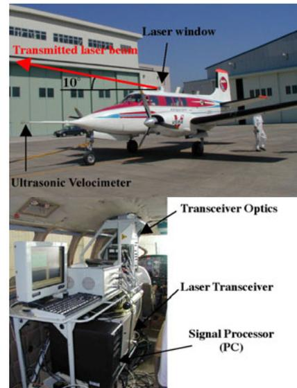
Fig. 2.4.1 Lidar installation on B65 research airplane.
