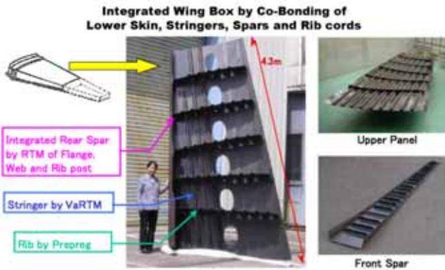
Fig 1 Co-bonded Wing Box
