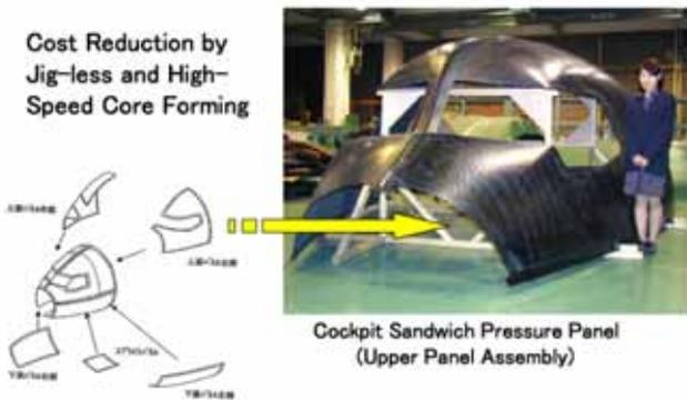
Fig.2 Cockpit Upper Sandwich Panel
