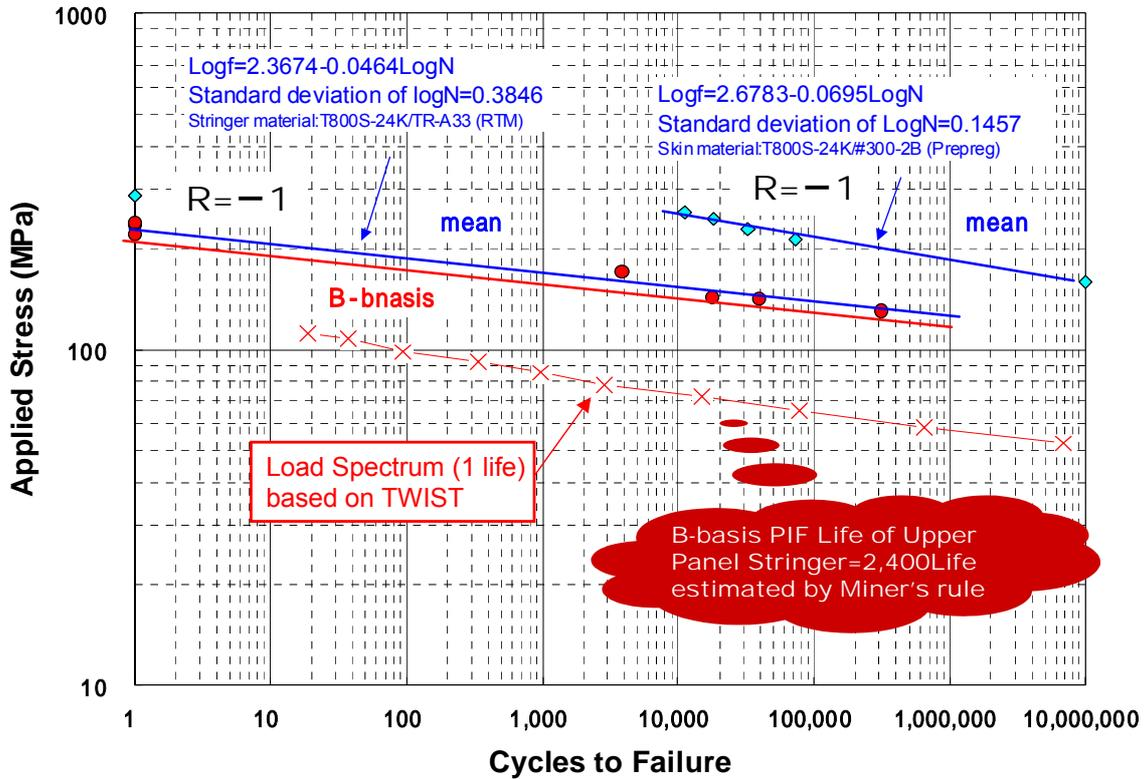
Fig.4 Post Impact Fatigue of Wing Upper Panel (PIF/BVID)
