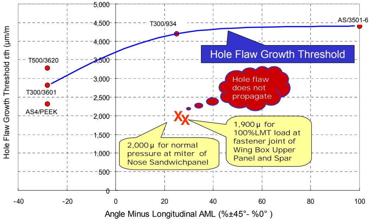
Fig.6 Hole Flaw Growth Threshold vs Working Strain
