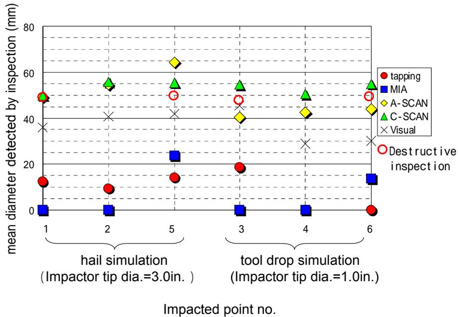
Fig.8 Comparison of NDI Detection Performance
