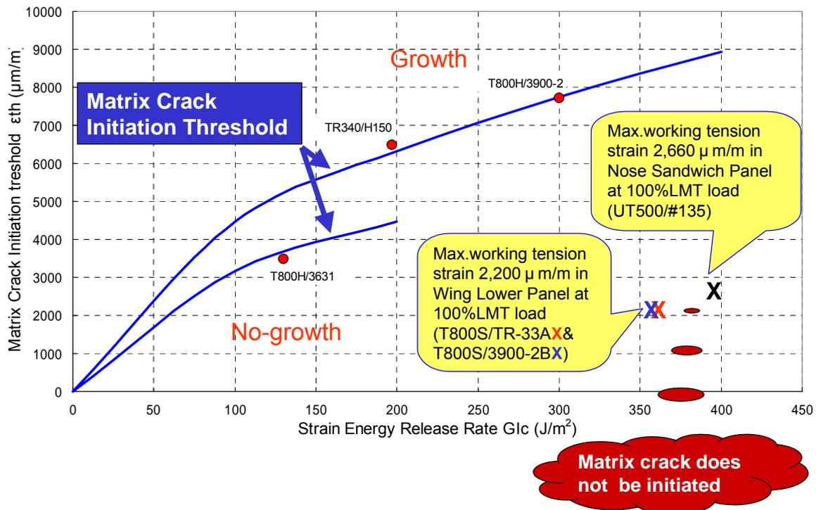
Fig.7 Matrix Crack Initiation Threshold vs Working Strain
