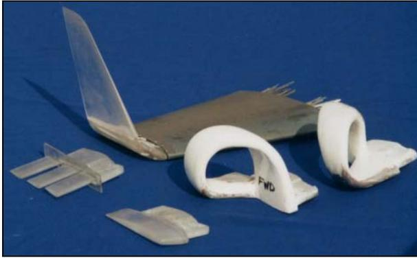
Fig. 3. The wing model including winglet shapes
