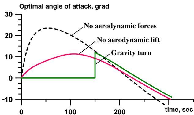
Fig. 2. The optimal time-programs of angle of attack of the launcher with zero effective lift.
