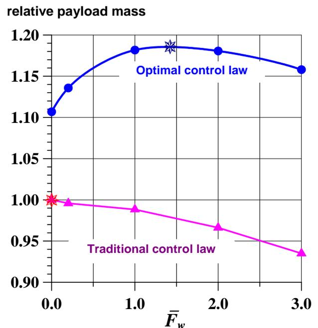
Fig. 13. Relative payload mass versus relative outer wing area  $\bar{F}_w$  of the launcher with defined engines and optimal initial mass.
