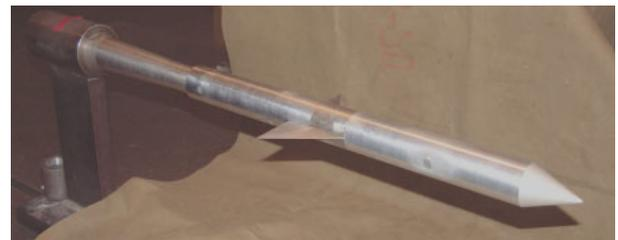
Fig.12. The winged-body aerodynamic model of a launcher in TsAGI's wind tunnel.
