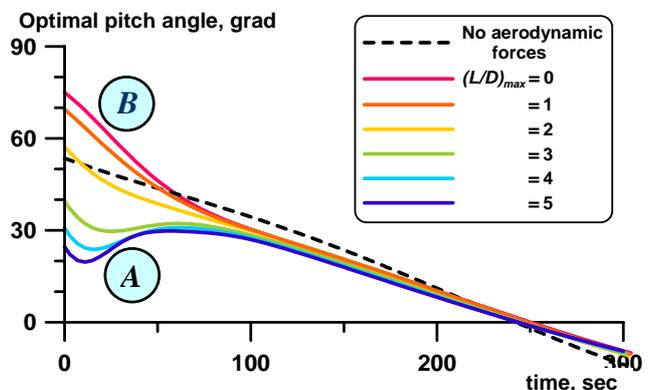
Fig. 4. Optimal time-programs of the pitch angle of the launcher with several lift-to-drag ratios,  $n_i = 1.4$ .
