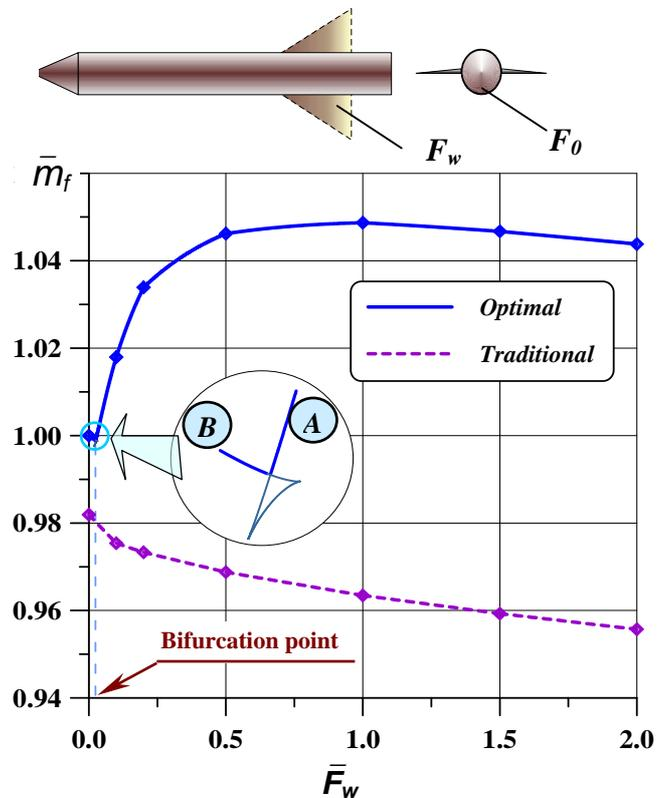
Fig. 10. The relative injected mass versus the relative outboard wing area for the winged cylindrical launcher. The bold line selects the global optimum.
