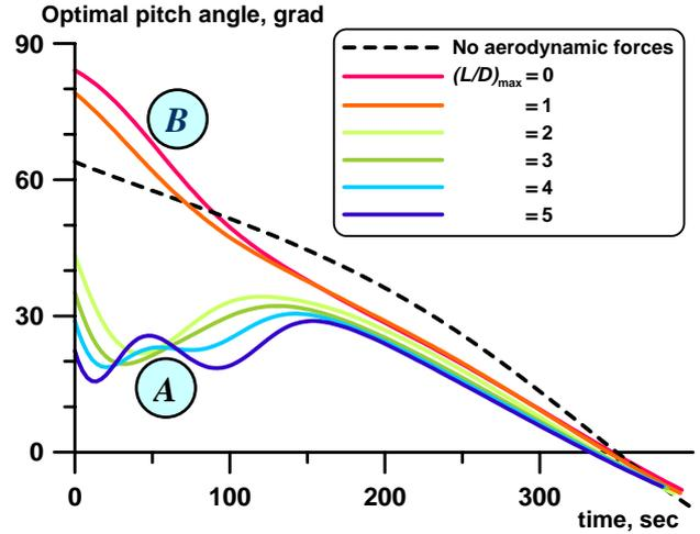
Fig. 6. Optimal time-programs of the pitch angle of the launcher with several lift-to-drag ratios,  $n_l = 1.04$ .
