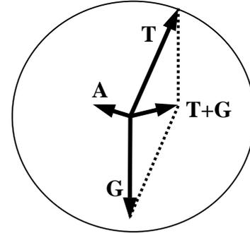
Fig. 1. The scheme of forces acting on a launcher.
