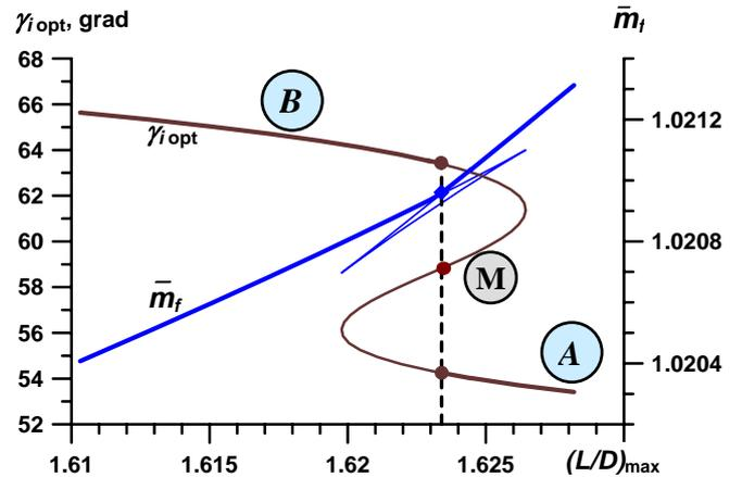
Fig. 7. Dependencies of the optimal initial path angle  $\gamma_{i\ opt}$  and relative injected mass  $\bar{m}_f$  on  $(L/D)_{max}$  of the launcher in the vicinity of the bifurcation point.
