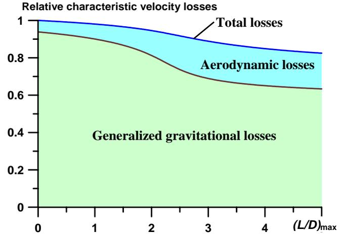
Fig. 3. Redistribution of characteristic velocity losses due to the maximum lift-to-drag ratio variation,  $n_i = 1.4$ .
