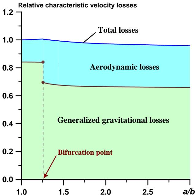
Fig. 9. Redistribution of characteristic velocity losses due to the contraction parameter variation of the conical launcher.
