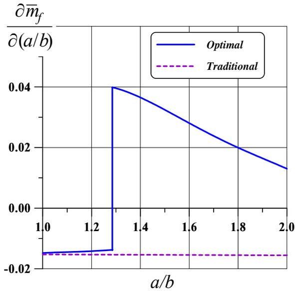
Fig. 11. The sensitivity coefficient versus the contraction parameter of the conical launcher.
