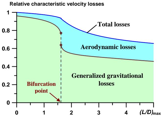
Fig. 5. Redistribution of characteristic velocity losses due to the maximum lift-to-drag ratio variation,  $n_l = 1.04$ .
