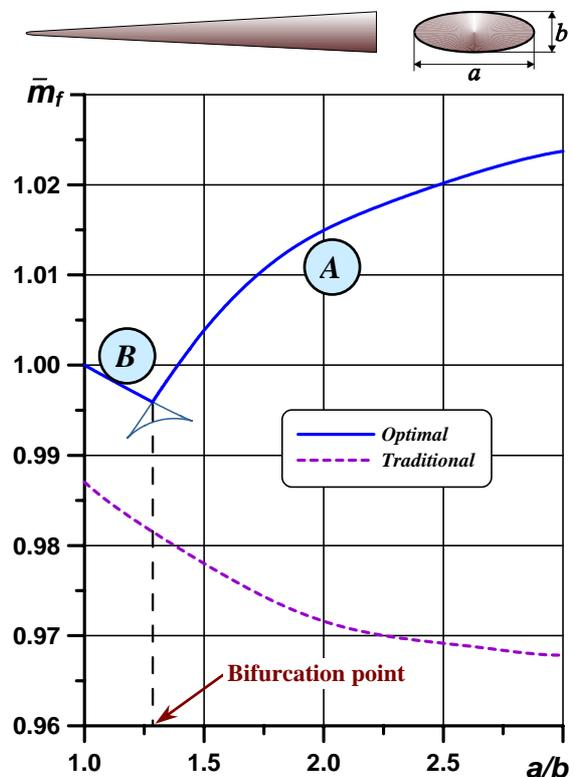
Fig.8. Relative injected mass versus contraction parameter of the conical launcher. The bold line selects the global optimum.
