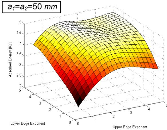
Fig. 8. Absorbed energy changing the exponents of the upper and lower edges –  $a_1=a_2=50 \text{ mm}$ .
