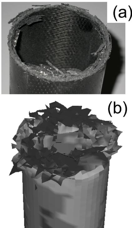
Fig. 2. Crashed cylinders, experiment (a) and numerical computation (b).
