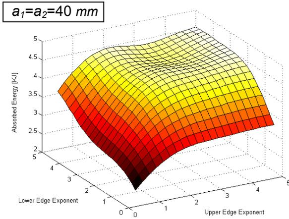
Fig. 7. Absorbed energy changing the exponents of the upper and lower edges –  $a_1=a_2=40 \text{ mm}$ .
