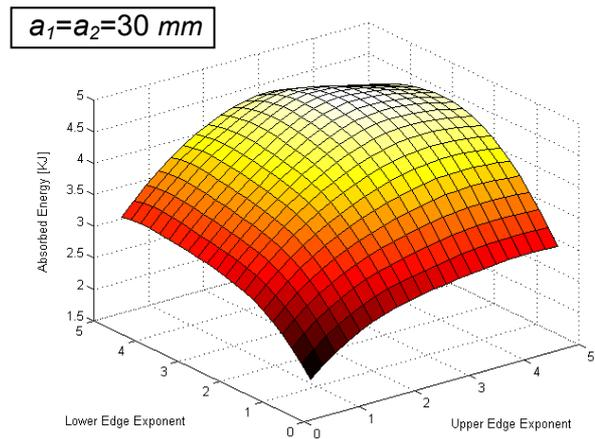
Fig. 6. Absorbed energy changing the exponents of the upper and lower edges –  $a_1=a_2=30$  mm.
