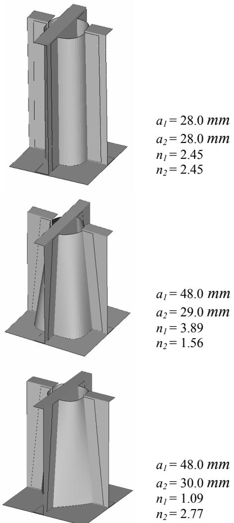
Fig. 4. Shapes of the stabilizer as a function of the design variables.
