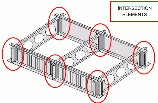
Fig. 1. A typical subfloor configuration.
