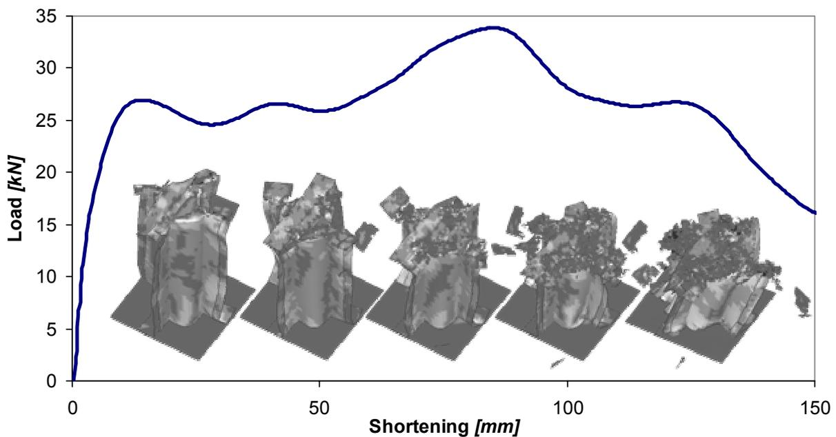
Fig. 10. Finite element behaviour of the third optimized configuration: load curve and deformed shape evolution.
