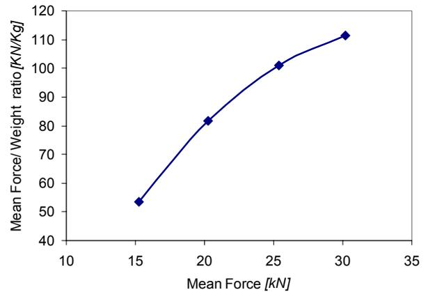
Fig. 9. Efficiency of the intersection elements vs. their mean force.
