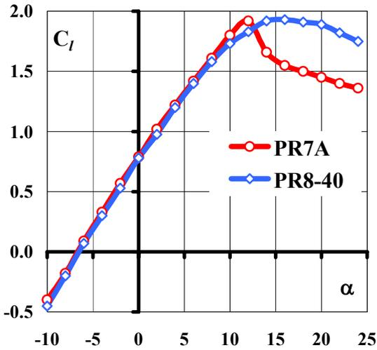
Fig. 7. Stall pattern of IAI high-lift airfoils, WT test,  $Re= 1.0 \cdot 10^6$ .
