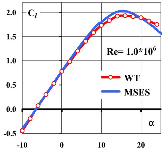
Fig. 11. Airfoil PR8-40 - lift curves, test-theory comparison.
