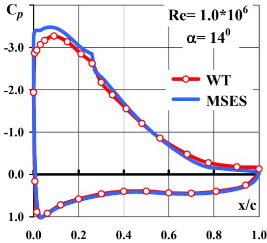
Fig. 13. Airfoil PR8-40 - pressure distributions, test-theory comparison.
