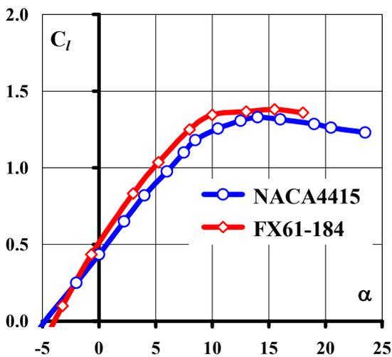
Fig. 5. Lift curves of mild stall airfoils, WT test,  $Re = 1.0 \cdot 10^6$ .
