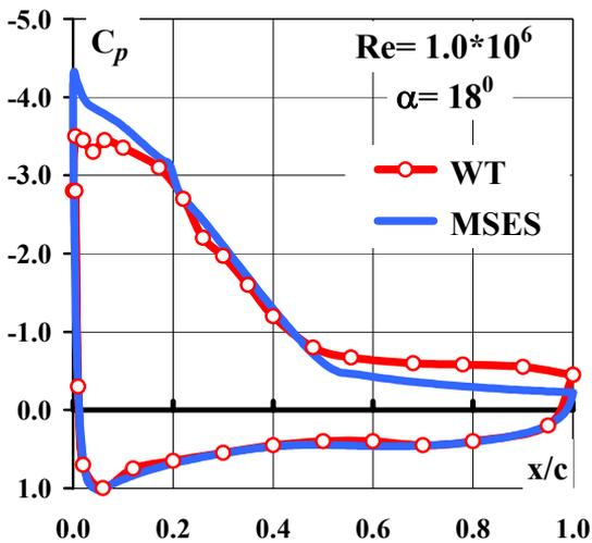
Fig. 14. Airfoil PR8-40 - pressure distributions, test-theory comparison.
