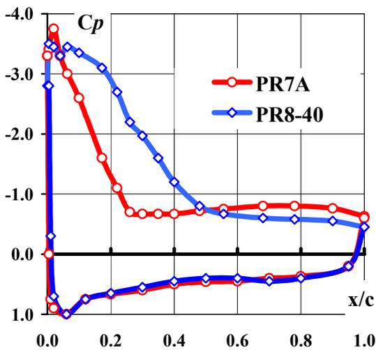
Fig. 9. Comparison of pressure distributions, WT test,  $Re=1.0 \cdot 10^6$ ,  $\alpha= 18^\circ$ .
