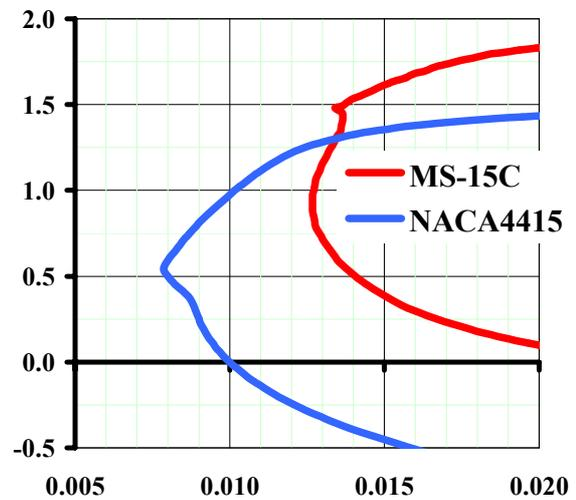
Fig. 22. Airfoil MS-15C vs NACA-4415, drag polars, MSES code,  $Re = 0.5 * 10^6$ .
