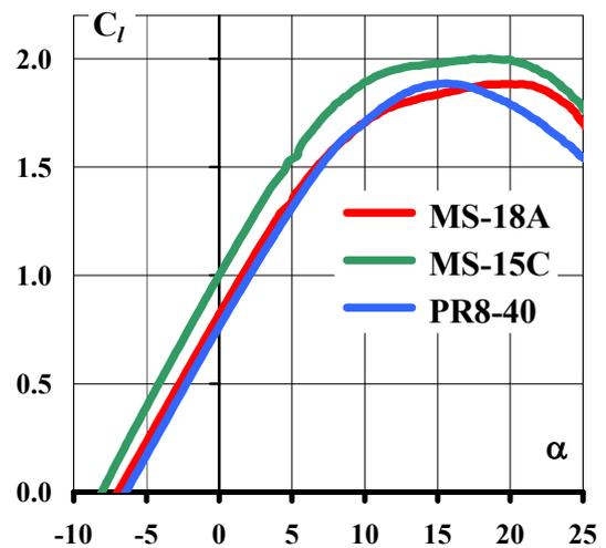
Fig. 16. Lift curves of MS-airfoils, MSES code,  $Re=0.5 \cdot 10^6$ .
