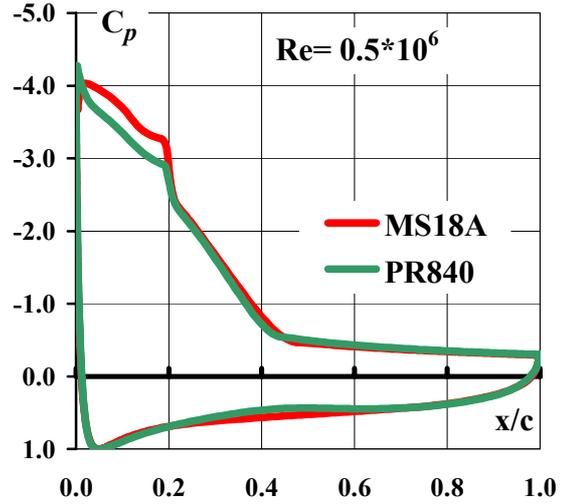
Fig. 20. Comparison of pressure distributions, airfoil MS-18A vs PR8-40,  $\alpha = 20^\circ$ .
