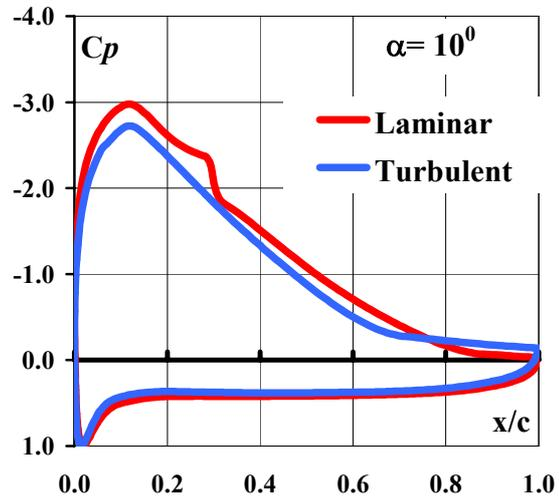
Fig. 26. Airfoil MS-18A - contamination effect, pressure distributions, MSES ,  $Re= 0.5 \cdot 10^6$ .
