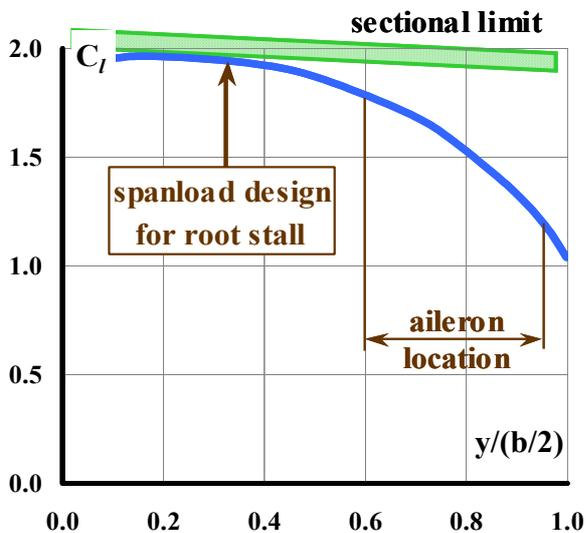
Fig. 28. Typical spanload distribution of moderate aspect ratio wing.
