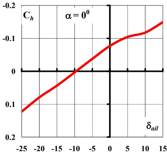
Fig. 32. Aileron hinge moments,  $Re= 1.0*10^6$ .
