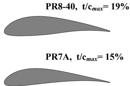
Fig 6. Airfoils PR8-40 and PR7A
