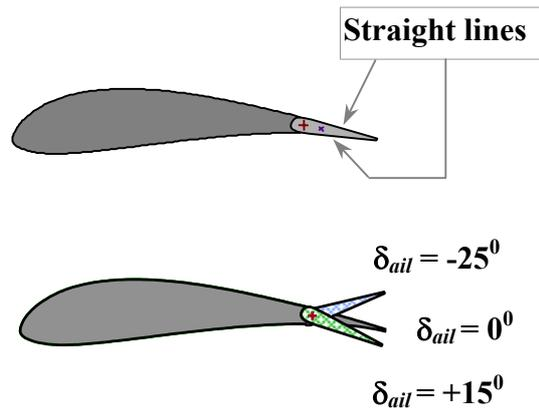
Fig. 29. Airfoil MS-18T – aileron definition.
