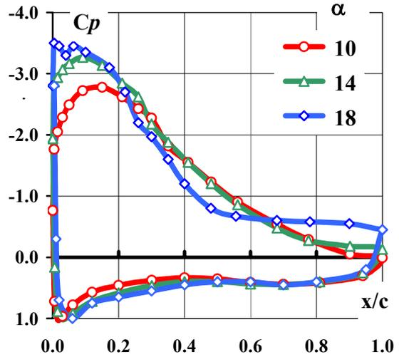
Fig. 10. Airfoil PR8-40 – development of trailing edge separation, WT test,  $Re= 1.0 \cdot 10^6$ .
