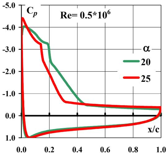
Fig. 18. Airfoil MS-18A – development of trailing edge separation.
