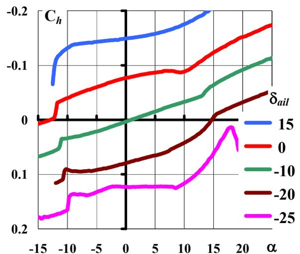
Fig. 31. Airfoil MS-18T - hinge moments, MSES code,  $Re= 1.0 \cdot 10^6$ .
