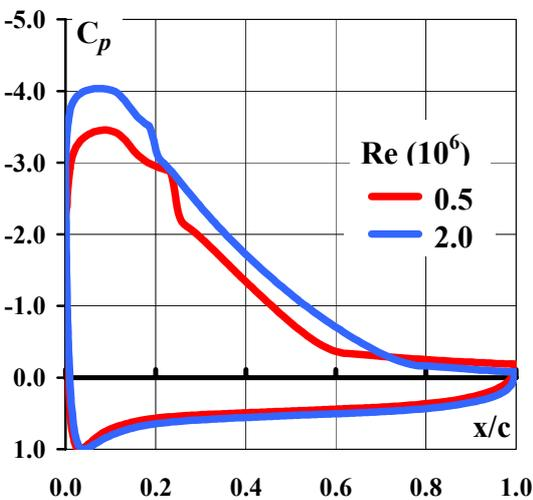
Fig. 24. Airfoil MS-18A – Reynolds effect, pressure distributions,  $\alpha= 15^{\circ}$ .
