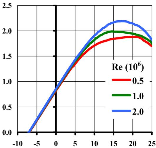
Fig. 23. Airfoil MS-18A - Reynolds effect, lift curves, MSES code.
