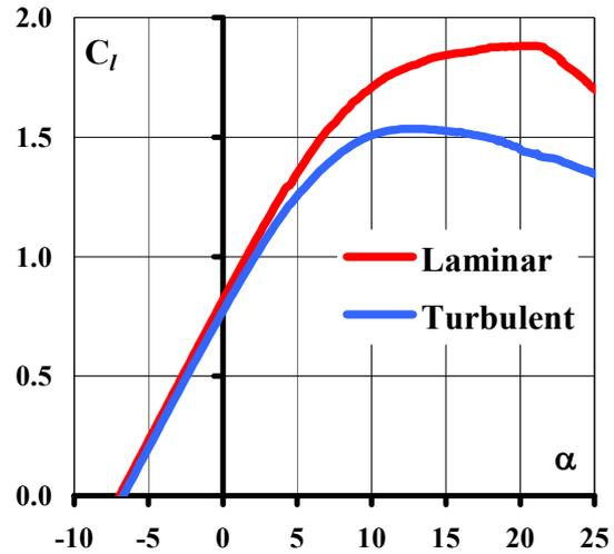
Fig. 25. Airfoil MS-18A - contamination effect, lift curves,  $Re= 0.5 \cdot 10^6$ .
