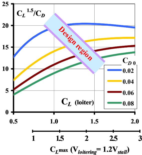
Fig. 2. Design region of UAV with moderate aspect ratio wings, AR= 12, e= 0.85.
