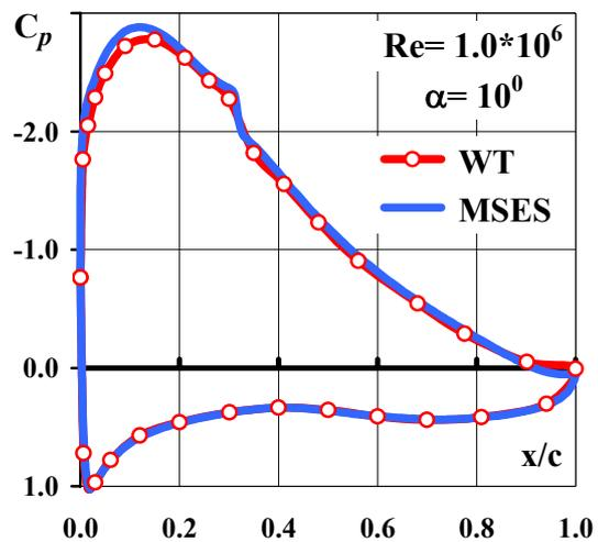
Fig. 12. Airfoil PR8-40 - pressure distributions, test-theory comparison.
