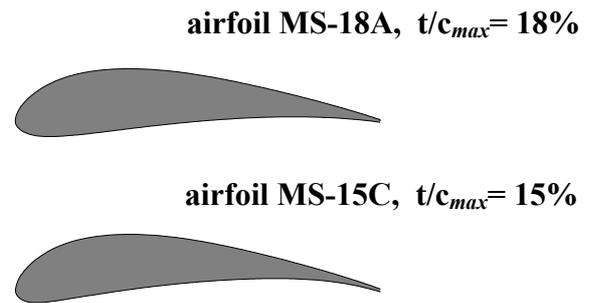
Fig. 15. High-lift, mild stall MS-airfoils.
