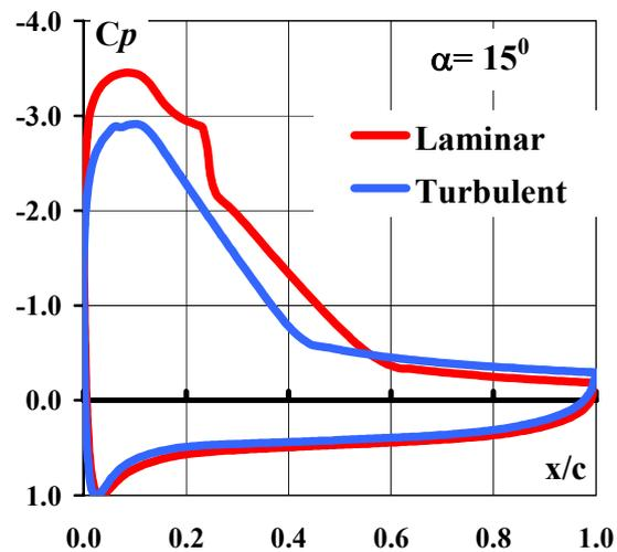
Fig. 27. Airfoil MS-18A - contamination effect, pressure distributions, MSES ,  $Re= 0.5 \cdot 10^6$ .
