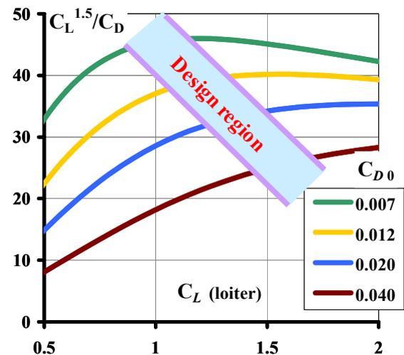
Fig. 1. Design region of UAV with high aspect ratio wings, AR= 25, e= 0.85.
