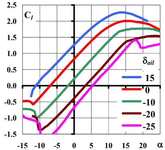
Fig. 30. Airfoil MS-18T - aileron deflections, MSES code,  $Re= 1.0 \cdot 10^6$ .
