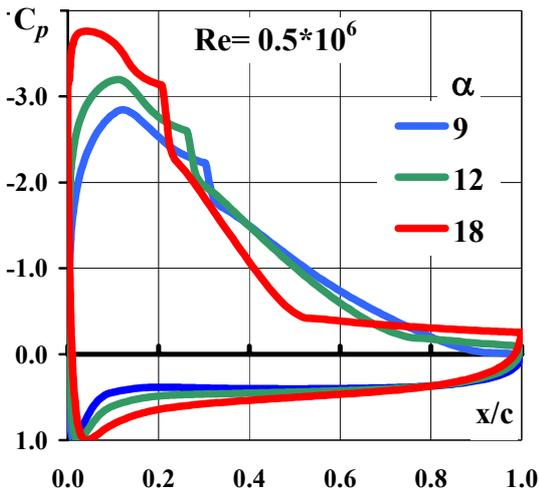
Fig. 17. Airfoil MS-18A – development of trailing edge separation.
