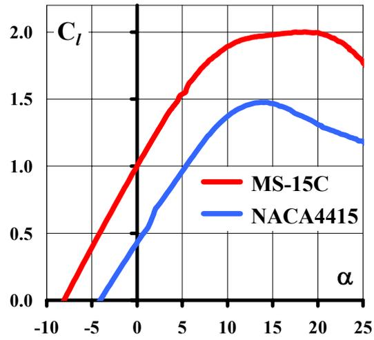
Fig. 21. Airfoil MS-15C vs NACA-4415, lift curves, MSES code,  $Re = 0.5 * 10^6$ .
