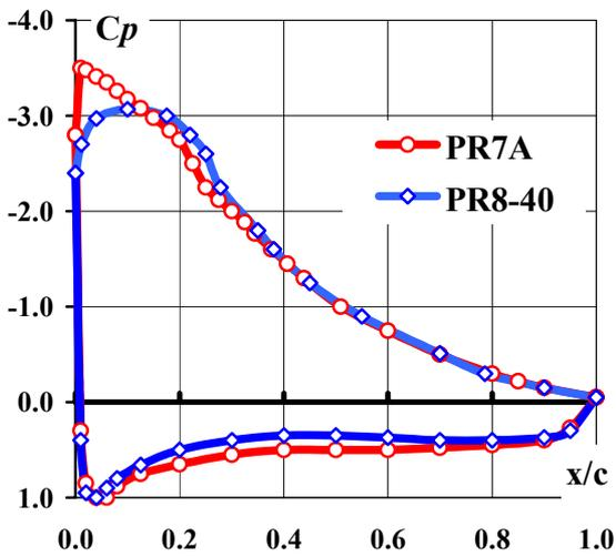
Fig. 8. Comparison of pressure distributions, WT test,  $Re=1.0 \cdot 10^6$ ,  $\alpha= 12^\circ$ .
