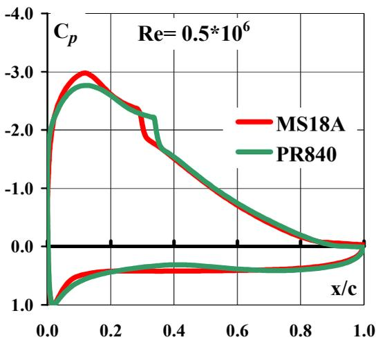
Fig. 19. Comparison of pressure distributions, airfoil MS-18A vs PR8-40,  $\alpha = 10^\circ$ .
