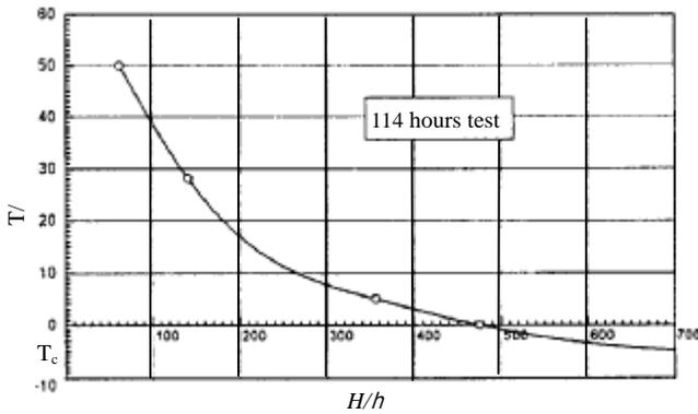
Fig. 1 T-H test curve of average corrosion up to 1 mm for Ly12cz aluminum alloy sheet
