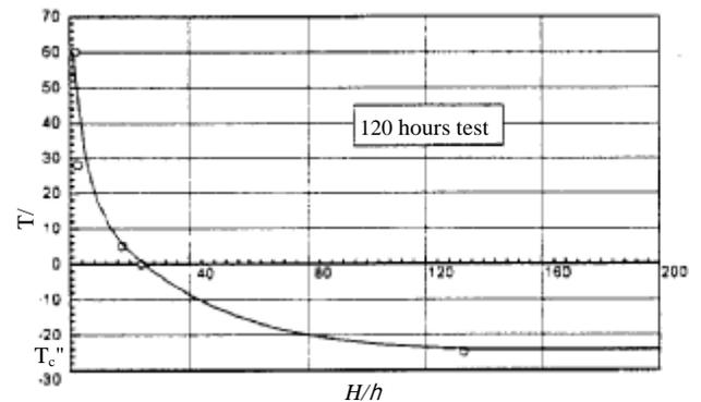
Fig. 3 T-H test curve of average corrosion up to 1 mg per square centimeter for 30CrMnSiA alloy steel sheet
