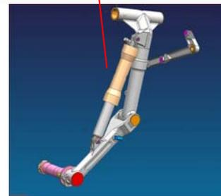
Fig. 4 – The main landing gear of VUT 100, new GA project of IAE
