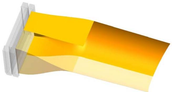
Fig. 22. Rear part of the by-pass cooling channel with the outlet accelerating nozzle
