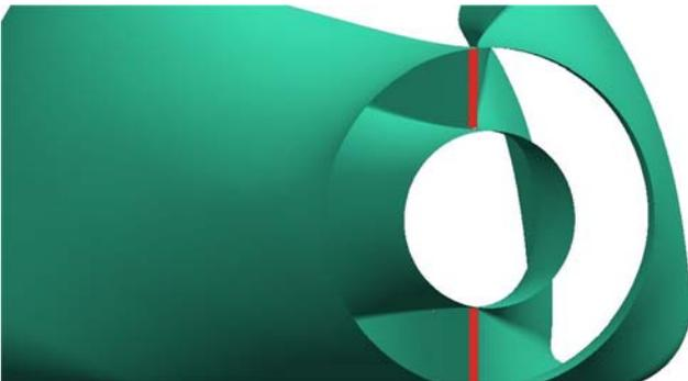
Fig. 18. Inlet channel with two slots (in red) for ventilation of the engine space by the suction
