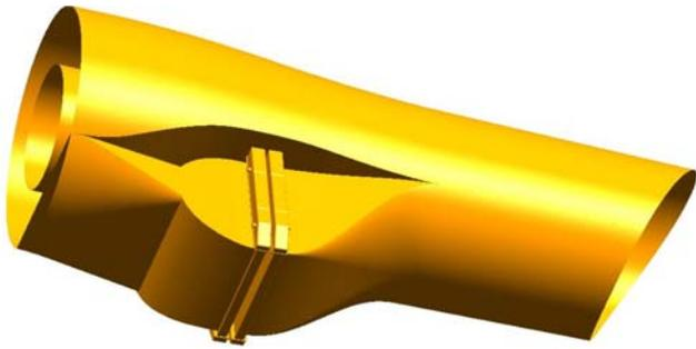
Fig. 23. Assembly of the jet pipe with the cooling channel
