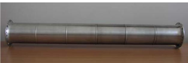
Fig. 26. Transmission shaft manufactured of the high strength aluminium alloy
