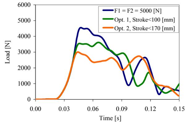
Fig. 9. Optimization results: lumbar spine load comparison between the optimized configurations and the initial one.
