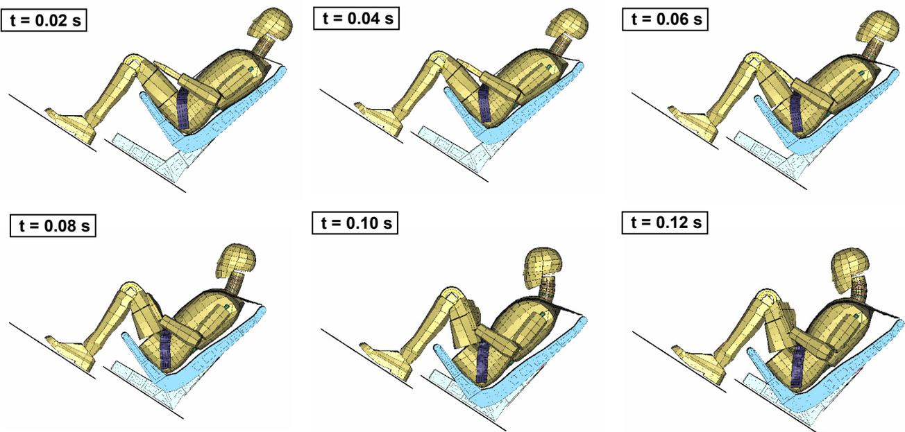
Fig. 10. Anthropomorphic dummy behavior for the optimized configuration of the absorbers with stroke of 170 mm.
