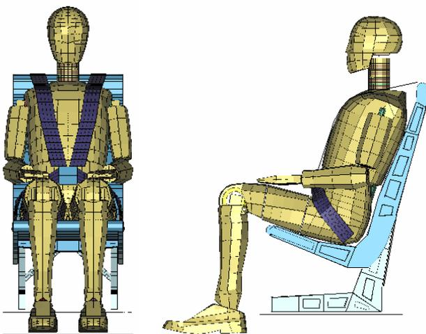
Fig. 2. Finite element model of seat and anthropomorphic dummy.
