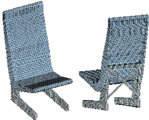
Fig. 1. Finite element model of the seat.
