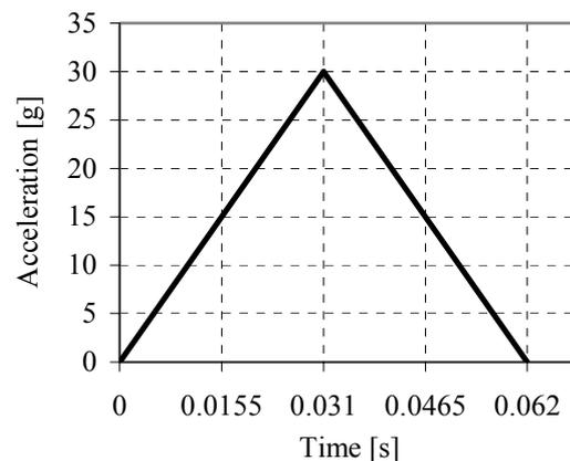
Fig. 3. Deceleration-time history for “Down Test” according to FAR/JAR specifications.
