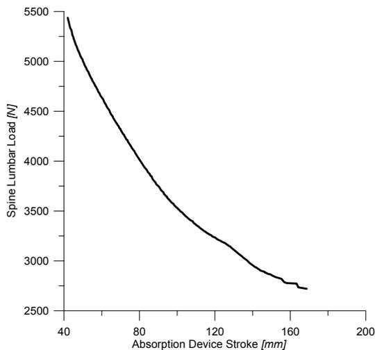
Fig. 8. Pareto set of the spine lumbar load vs. the absorption device stroke.
