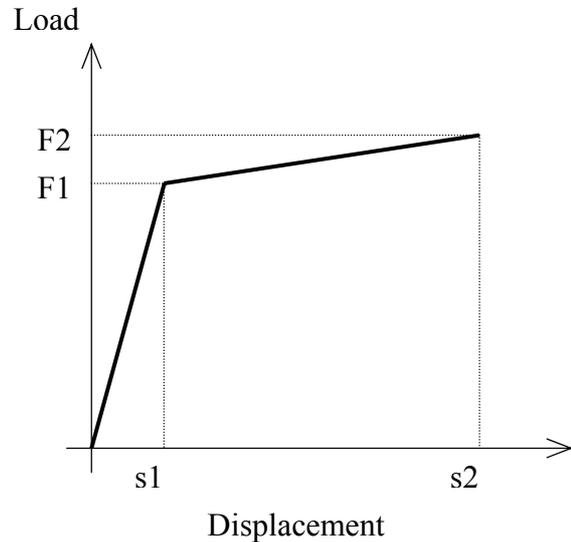
Fig. 5. Force-Displacement curve of the energy absorbers.
