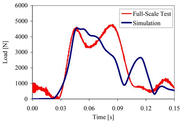
Fig. 4. Lumbar spine load time history, comparison between full-scale test and numerical simulation.
