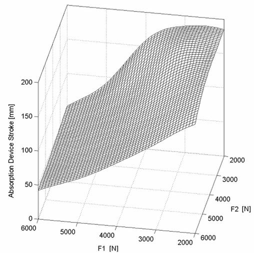
Fig. 7. Response surface of the absorption device stroke.
