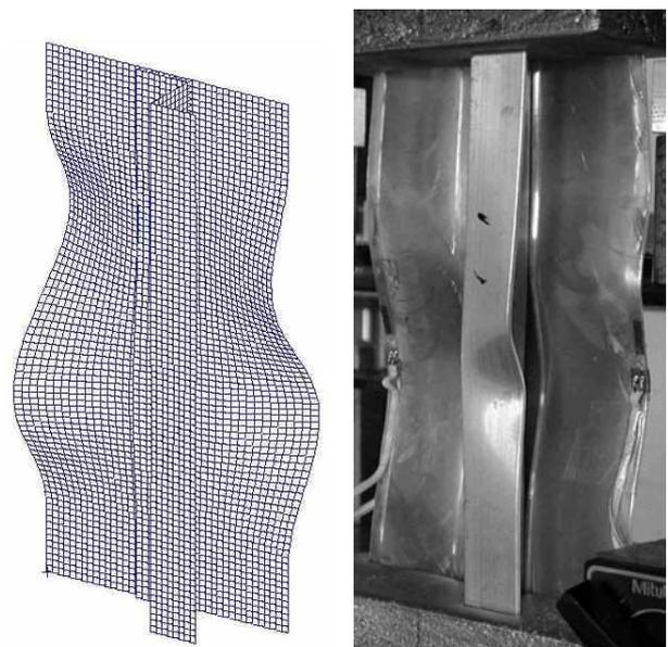
Fig. 8. FE Method 3 predicted failure mode and test specimen 2 failure mode
