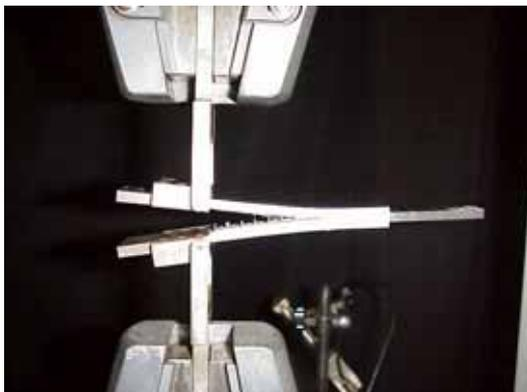
Fig.4. A picture of DCB test
