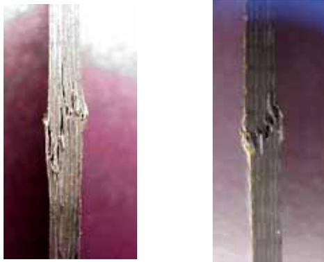
Fig. 18. Pictures of side views of OHC specimen after compression test
