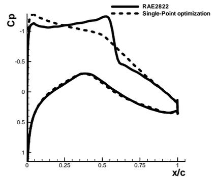
Fig.1 The comparison of pressure distributions
