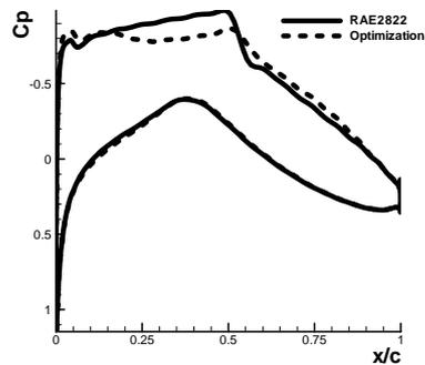
Fig.4 The comparison of pressure distributions on point 2)
