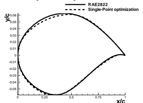
Fig.2 The comparison of geometries
