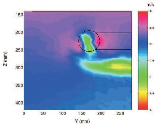
**Fig. 19** Distribution of axial velocity Winglet off at  $3c \alpha = 8^\circ$
