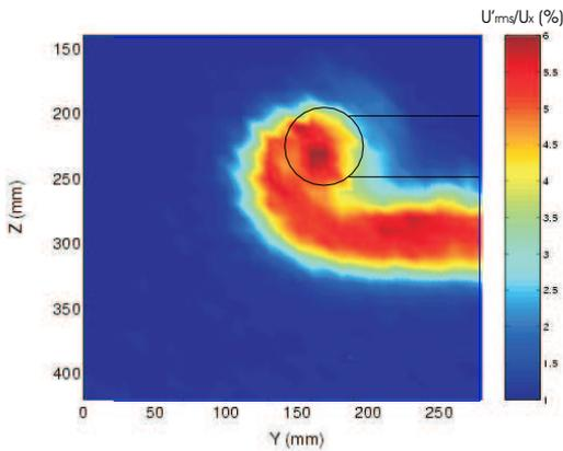
**Fig. 15** Intensity of the turbulence Winglets off
