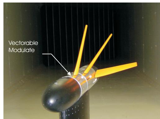
**Fig. 1** Cylindrical modules at the tip-tank
