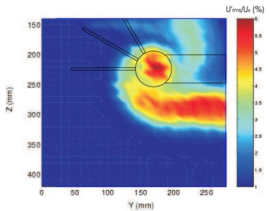
**Fig. 17** Intensity of the turbulence  $60^\circ A, 30^\circ B, 0^\circ C$  at  $3c \alpha = 8^\circ$
