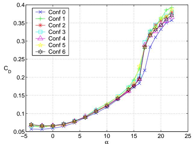
**Fig. 9** Coefficient drag curves
