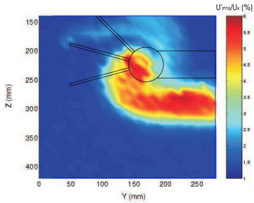
**Fig. 18** Intensity of the turbulence  $45^\circ A, 15^\circ B, -15^\circ C$  at  $3c \alpha = 8^\circ$
