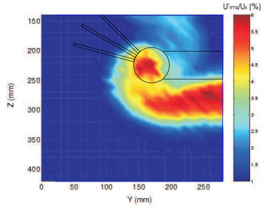
**Fig. 16** Intensity of the turbulence  $45^\circ A, 30^\circ B, 15^\circ C$  at  $3c \alpha = 8^\circ$
