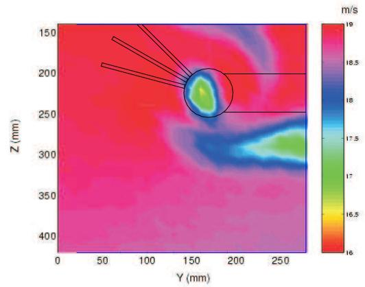
**Fig. 20** Distribution of axial velocity  $45^\circ A, 30^\circ B, 15^\circ C$  at  $3c \alpha = 8^\circ$
