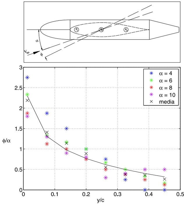
Fig. 4 Local flow direction 0.375c
