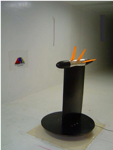
**Fig. 2** Model inside the wind tunnel
