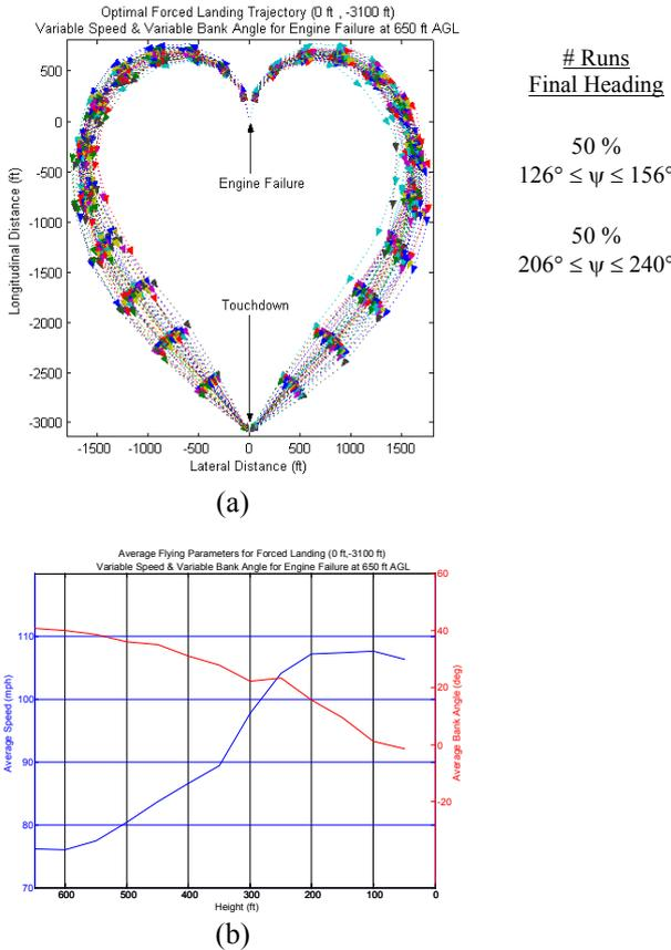
Fig. 7. Optimal Forced Landing (0 ft, -3100 ft) Continuous Speed and Continuous Bank Angle at 650 ft AGL
