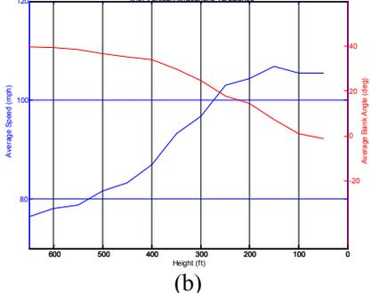
Fig. 10. Optimal Forced Landing (0 ft, -3100 ft) Continuous Speed and Continuous Bank Angle at 650 ft AGL with Vertical Atmospheric Turbulence
