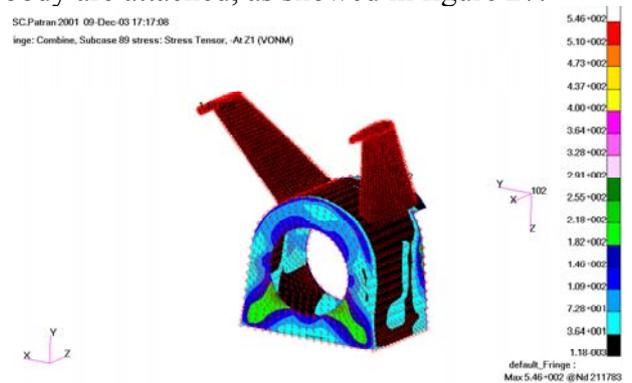
Fig. 25: stress tensor values on the most rear frame doubled
