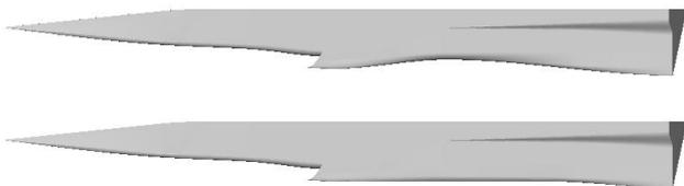
**Fig. 14. Two studied alternatives for rear fuselage geometry.**
